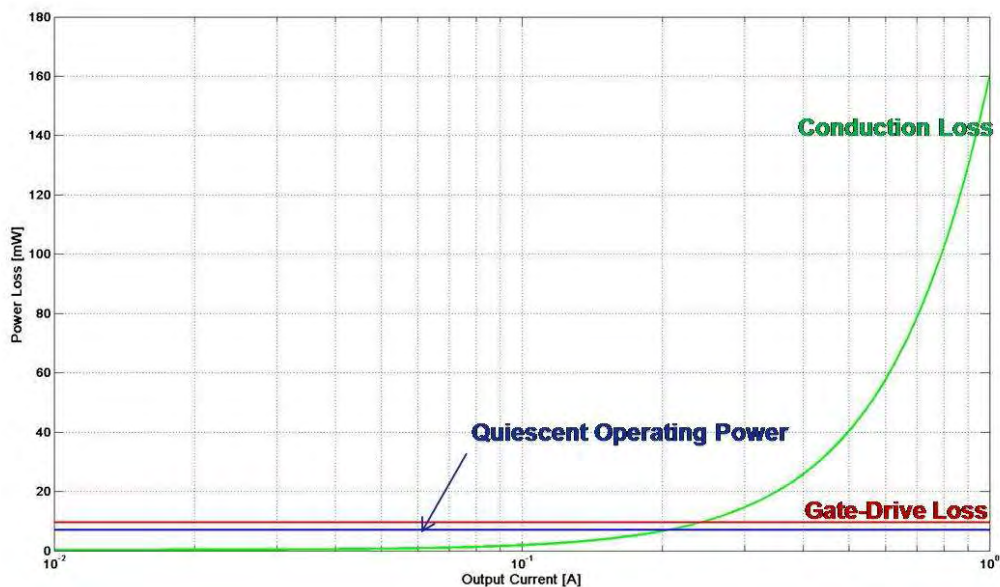
Fig. 1.15: Estimated conduction losses, gate-drive losses and quiescent operating power versus output current in the range 10mA→1A for a PWM buck.
