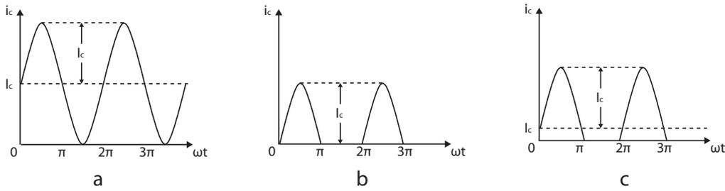
Figure 2.2: Bias current of transistor operating in: a – Class-A, b – Class-B, c – Class-AB amplifier stages
