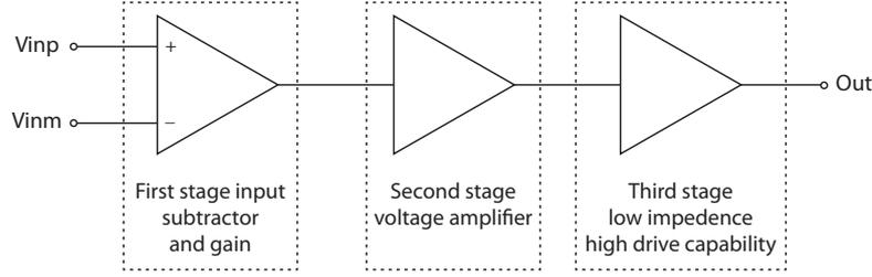
Figure 2.1: A general three-stage amplifier structure
