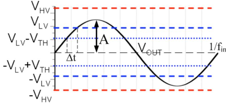
Figure 2.7: Output voltage versus time: supply voltage rails and switching point levels
