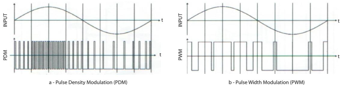
Figure 2.12: Pulse modulations examples: a – PDM, b – PWM
