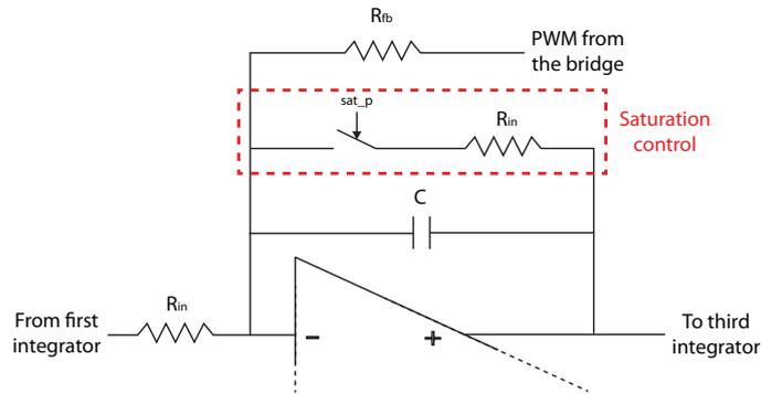
Figure 3.18: Saturation control implementation on the second integrator
