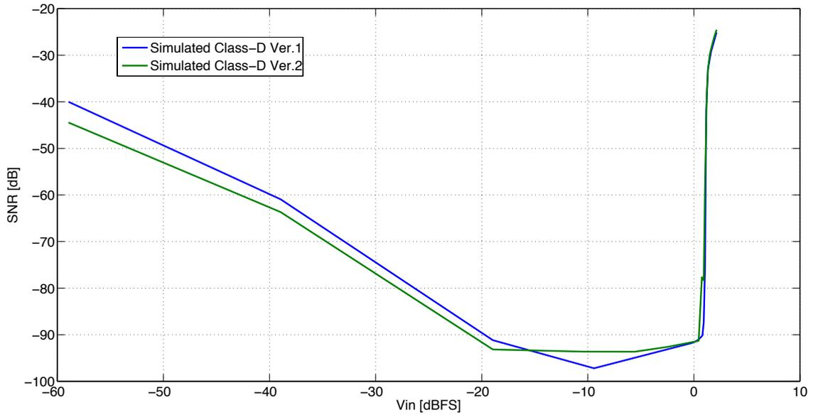
Figure 3.20: Comparison between the THD performance of Ver. 1 and Ver. 2 third-order Class-D amplifiers (input signal full-scale = 1.32 V)
