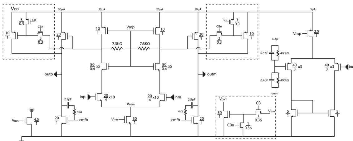
Figure 3.16: Ver. 2 opamp for the second and third integration stages, based on a fully differential Class-A architecture
