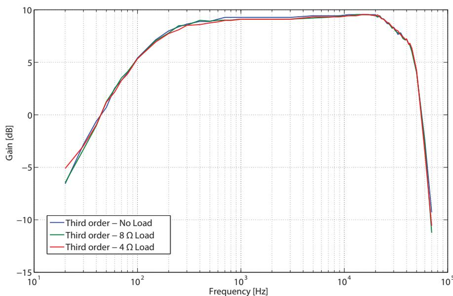
Figure 3.14: AC-coupled transfer function of third-order Class-D amplifier
