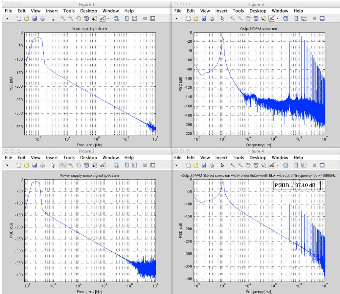
Figure A.12: PSRR analysis – Output data
