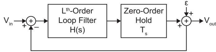
Figure 2.25: Linearized equivalent circuit of a  $\Sigma\Delta$  modulator or a class-D amplifier
