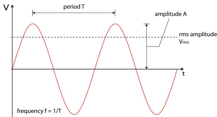
Figure 1.2: Sine-wave time behavior
