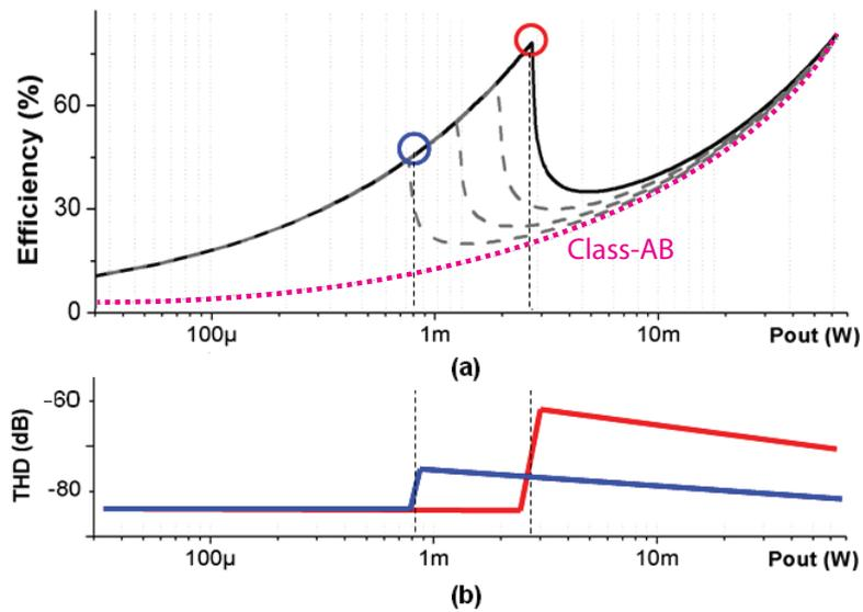
Figure 2.10: Class-G amplifier: a – Efficiency, b – THD versus output power at different switching point level
