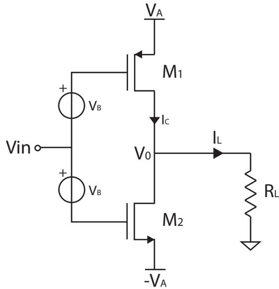
Figure 2.5: General Class-AB schematic
