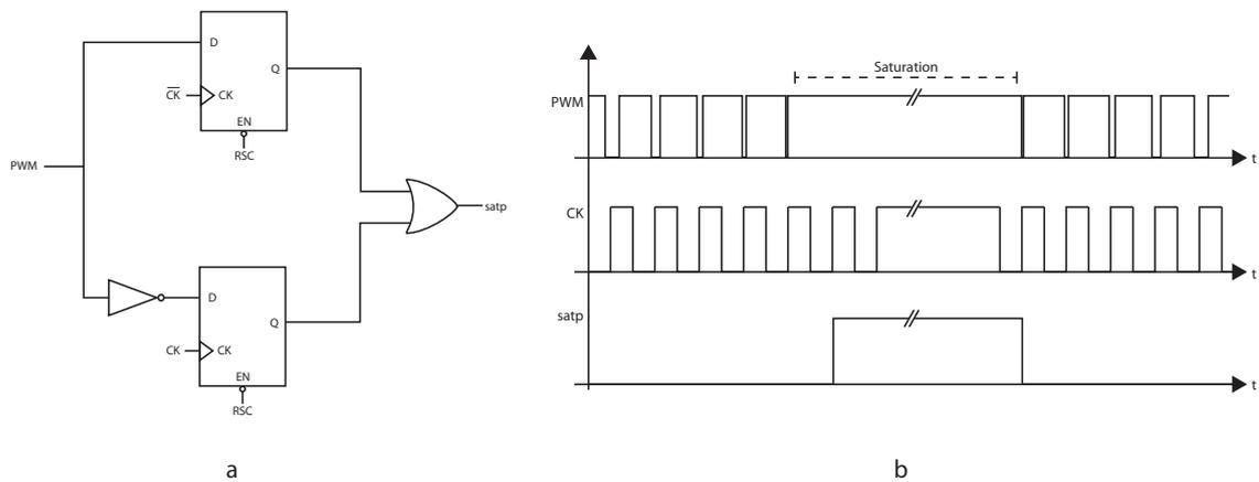
Figure 3.19: Saturation control logic: a – Schematic, b – Signal behavior
