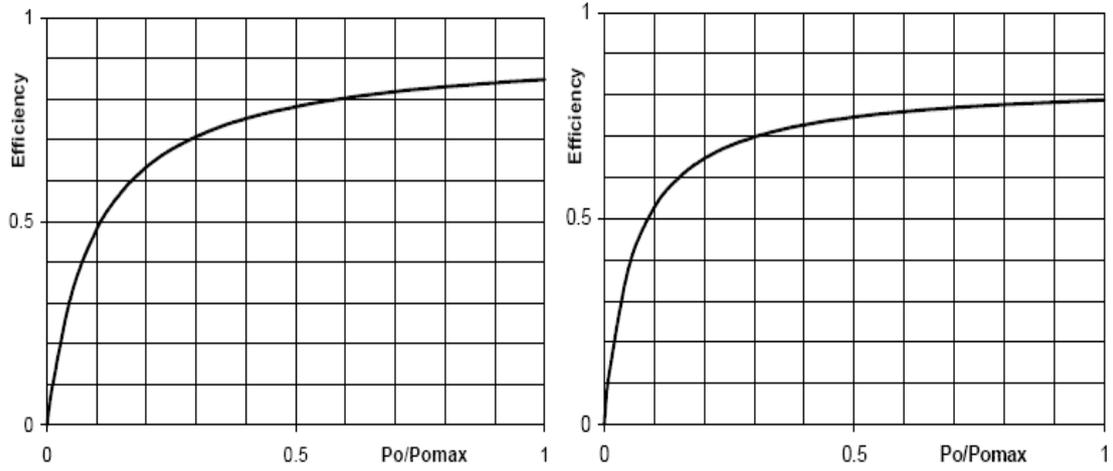
Figure 1.5: Simulated efficiency of two hypothetical audio amplifiers with different quiescent and maximum dissipations (linear scale)
