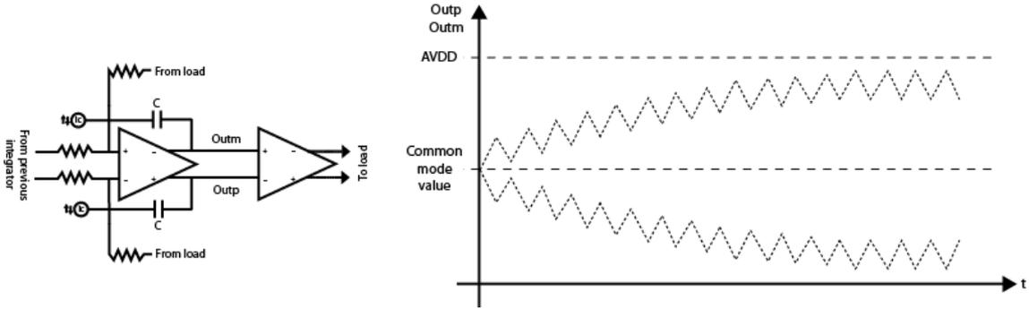
Figure 3.7: Integrator output behavior in the presence of carrier offset
