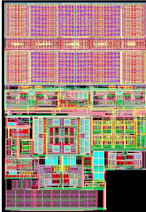
Figure 3.22: Layout of the third-order Class-D amplifier Ver. 2
