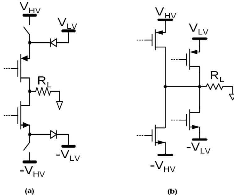
Figure 2.8: Class G topologies: a – Serial and b – Parallel
