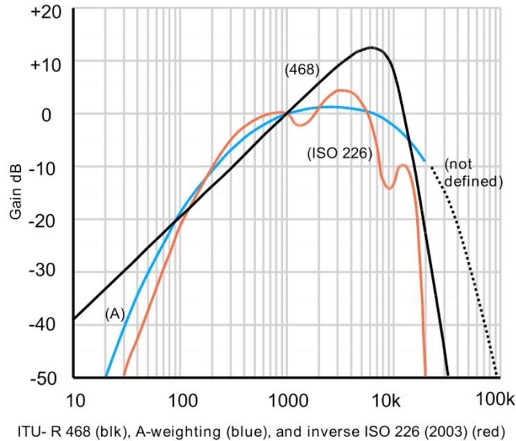
Figure 1.1: Weighting curves: ITU-R 468 in black, A-weighting in blue and inverse ISO 226 in red
