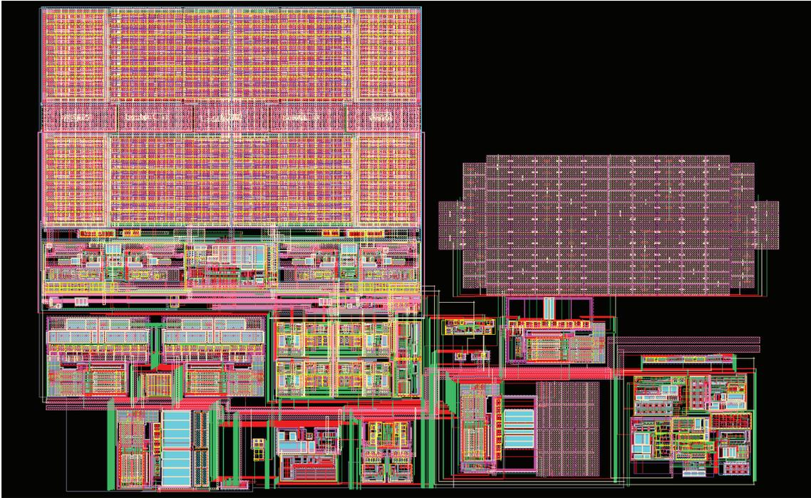
Figure 3.11: Third-order Class-D amplifier layout
