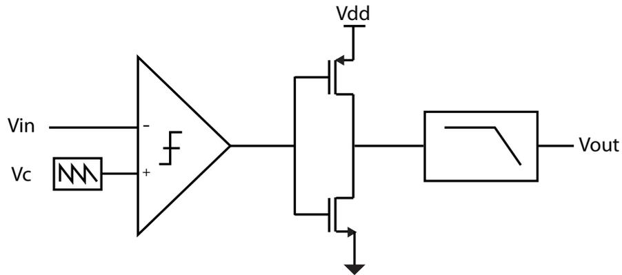
Figure 2.19: Single-ended open-loop Class-D amplifier implementation
