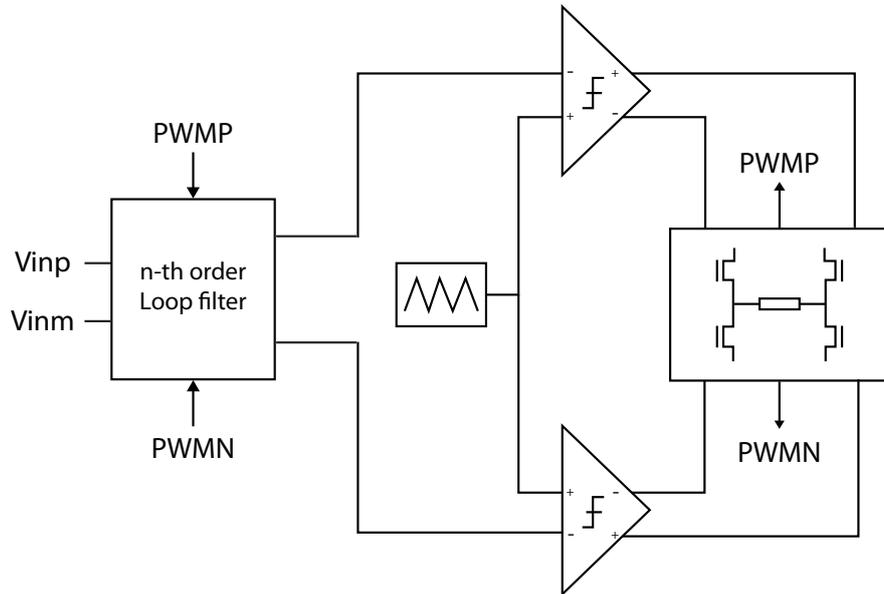
Figure 2.23: High-order fully-differential closed-loop Class-D amplifier implementation
