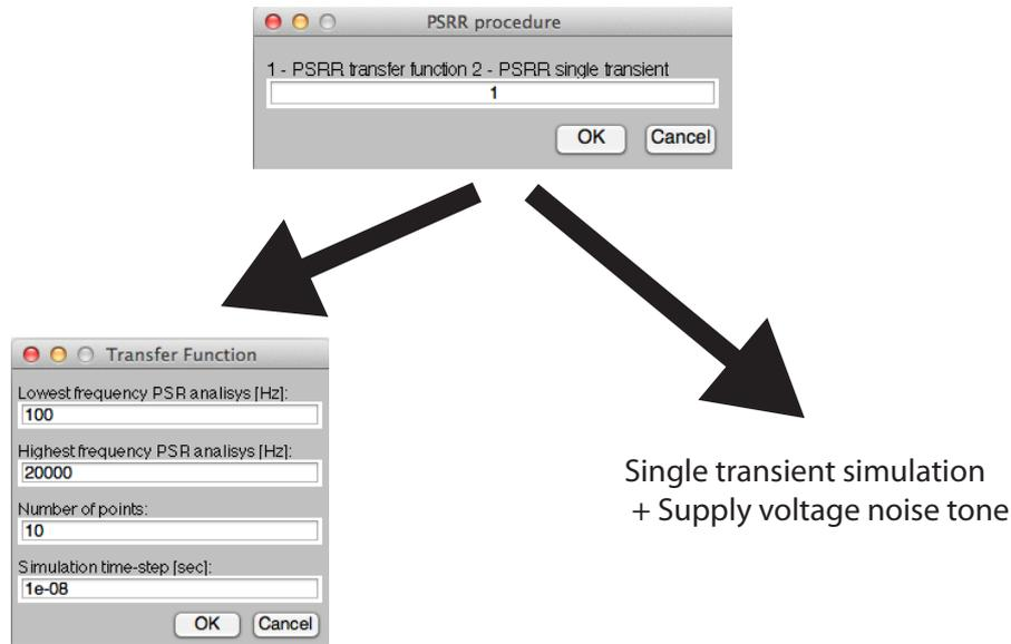
Figure A.11: PSRR analysis – Input settings menu
