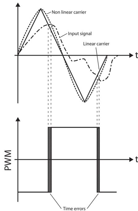
Figure 2.18: Time errors due to carrier non-linearity
