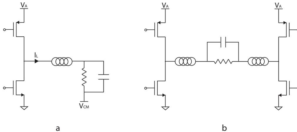
Figure 2.15: Possible output power stage architectures: a – Half-bridge, b – Full-bridge (BTL)
