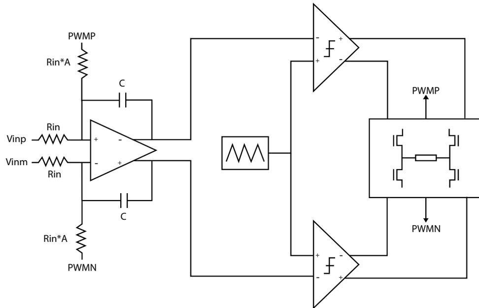
Figure 2.21: Fully-differential closed-loop Class-D amplifier implementation with BTL power stage
