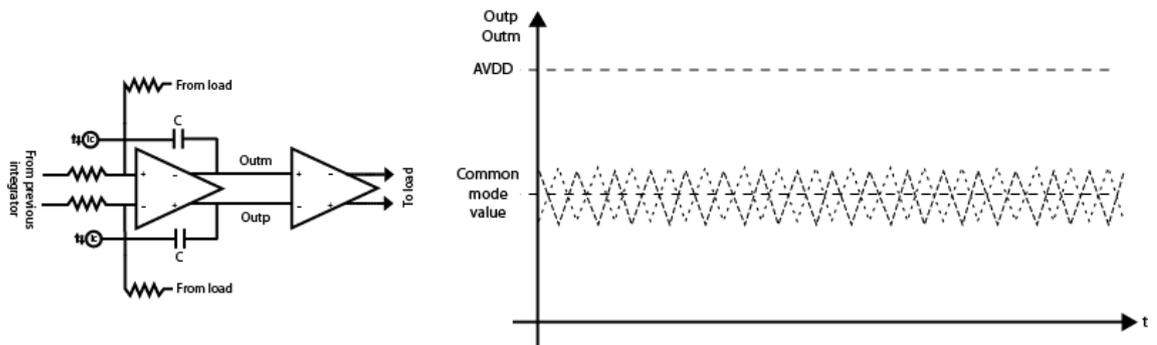
Figure 3.9: Integrator output behavior in the presence of carrier offset with the offset control circuit
