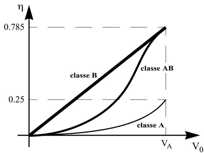
Figure 2.6: Comparison between theoretical efficiency curves
