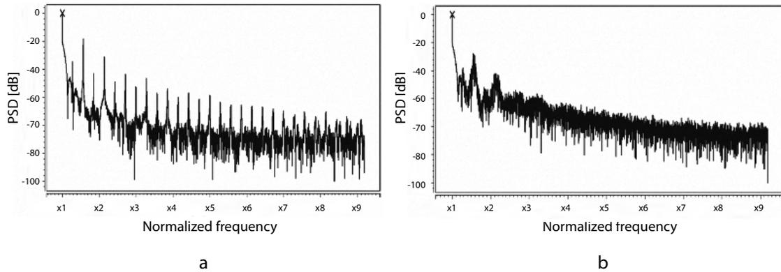
Figure 1.9: Example of a general Class-D spectrum at high frequencies: a – Without EMI control system, b – With EMI control system
