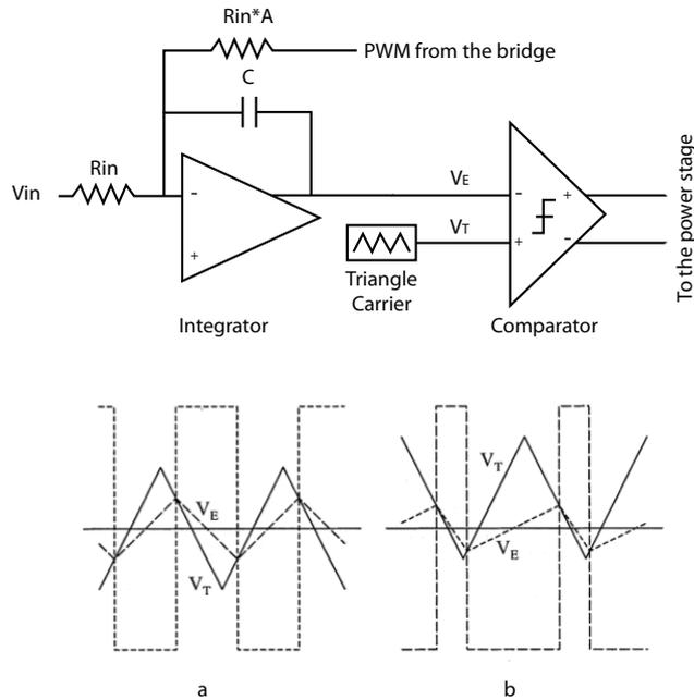
Figure 2.27: Internal loop signals: a – Zero input, b – Positive input
