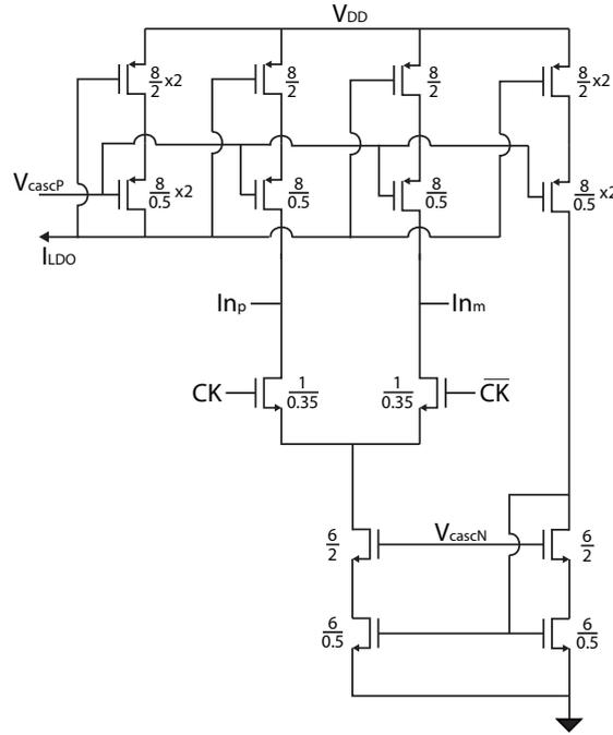
Figure 3.5: Carrier insertion circuit detailed schematic
