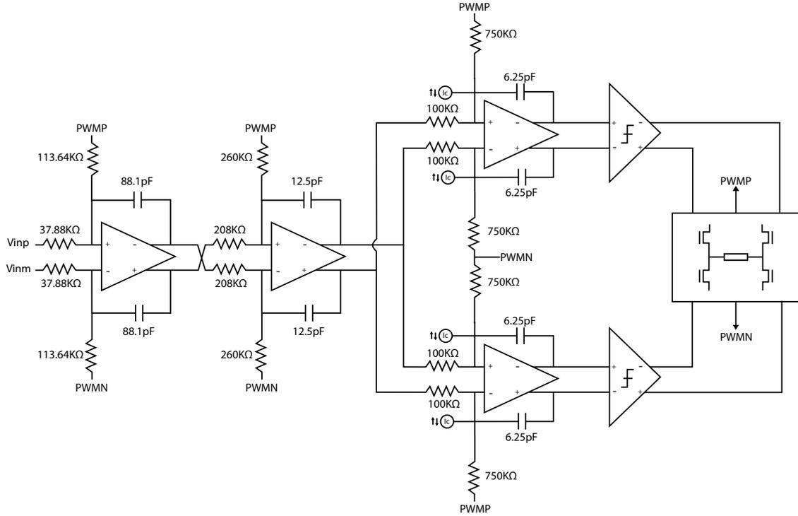
Figure 3.2: Third-order Class-D amplifier schematic
