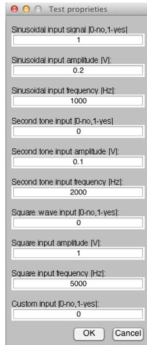
Figure A.5: Transient analysis – Input settings menu
