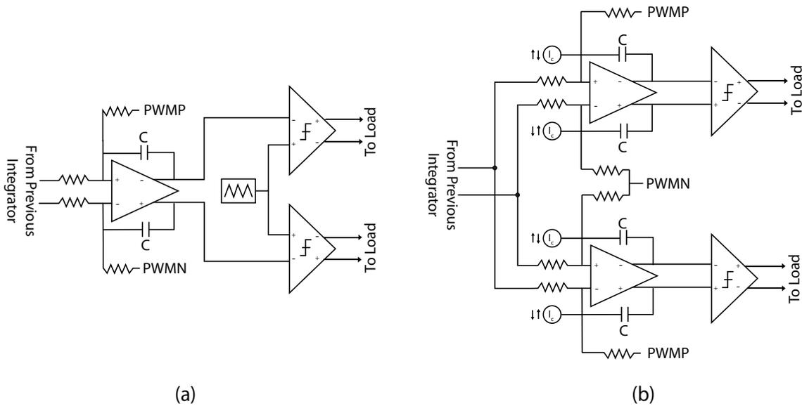
Figure 3.3: Carrier insertion: a – Stand alone generator, b – Square wave injection
