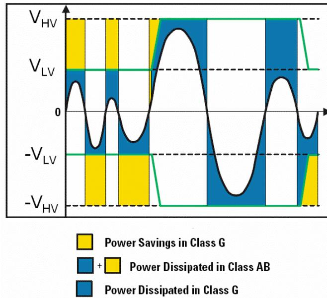
Figure 2.9: Intuitive view of the Class-G efficiency improvement with music as input signal
