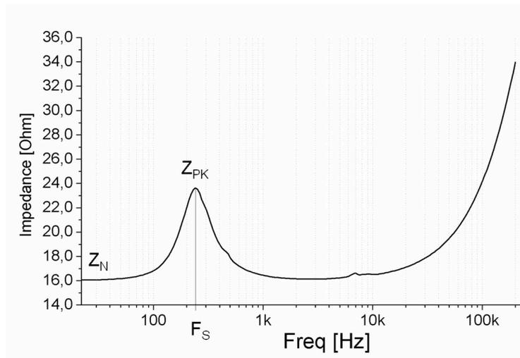
Figure 1.7: Module of the electrical impedance of a general speaker versus frequency
