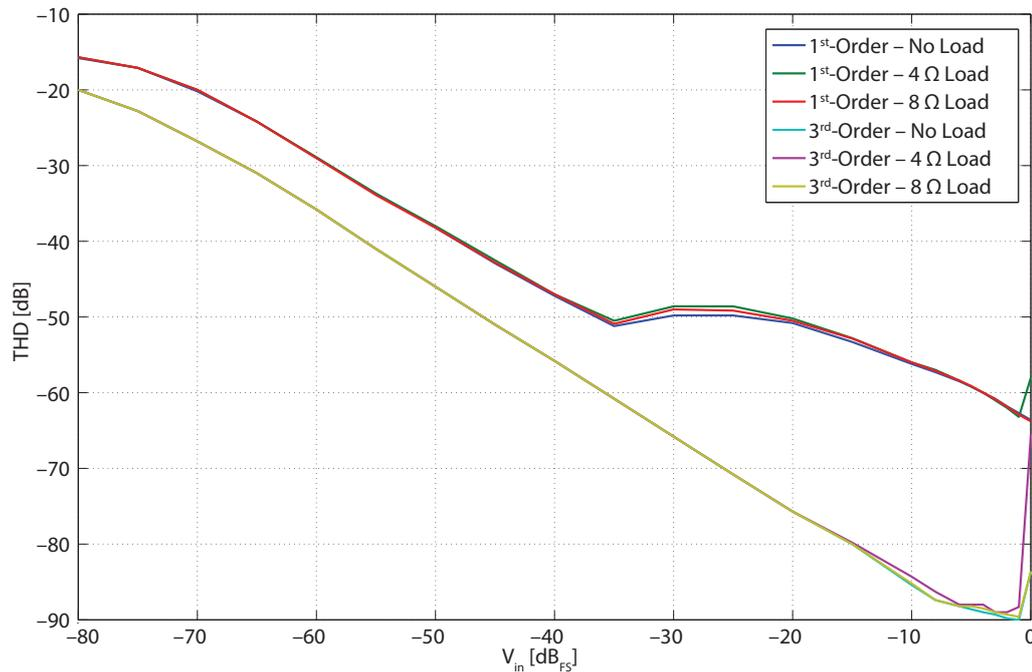
Figure 3.13: THD as a function of input signal level: comparison between first and third-order Class-D amplifier
