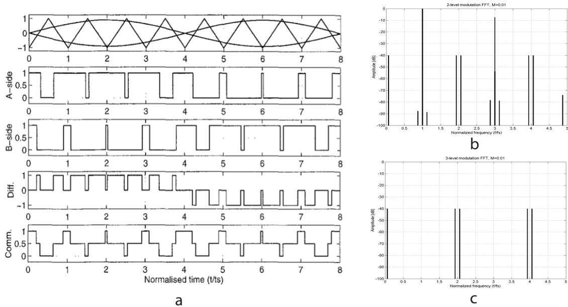
Figure 2.16: Three level PWM: a – Signals behavior, b – Two-level PWM spectrum, c – Three-level PWM spectrum
