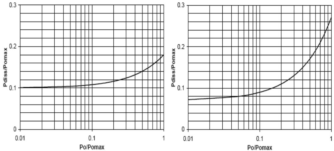
Figure 1.6: Simulated efficiency of two hypothetical audio amplifiers with different quiescent and maximum dissipations (logarithmic scale)
