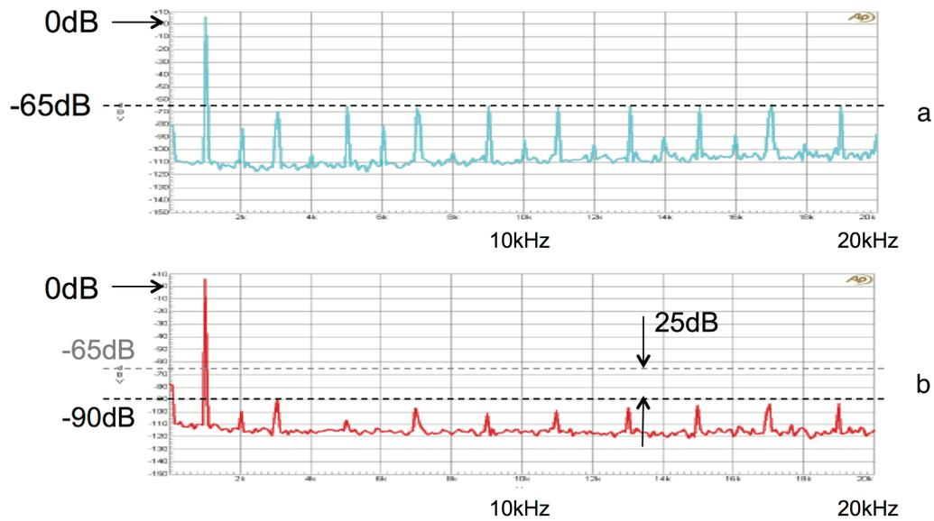
Figure 3.12: Comparison between output spectra with  $V_{in} = -3 \text{ dB}_{FS}$  of: a – First-order amplifier, b – Third-order amplifier
