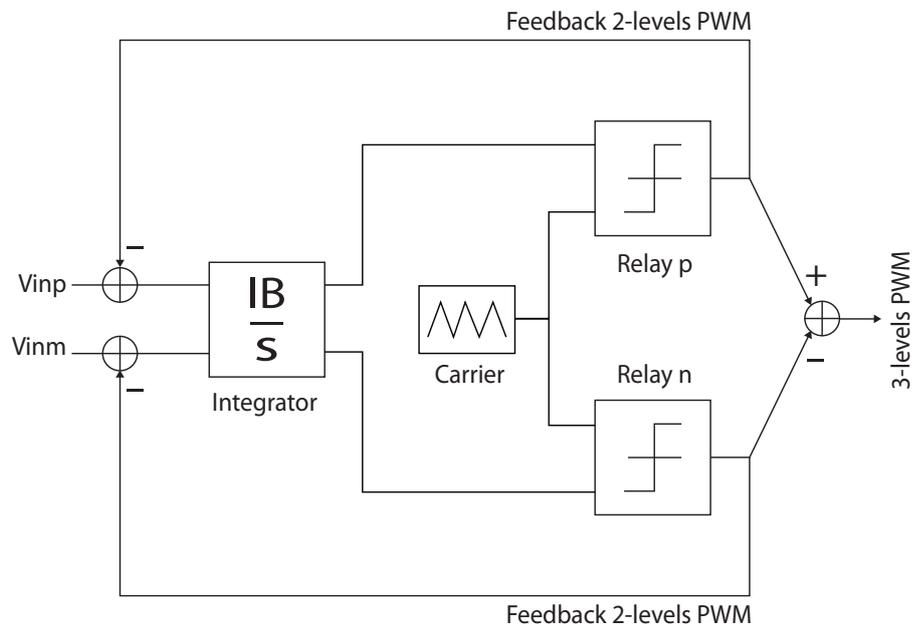
Figure 2.22: Fully-differential closed-loop Class-D amplifier model
