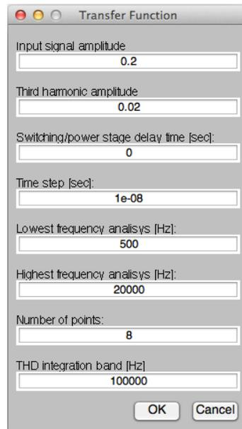
Figure A.8: Transfer function analysis – Input settings menu
