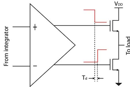
Figure 2.17: Dead-time control in power bridge driver signals
