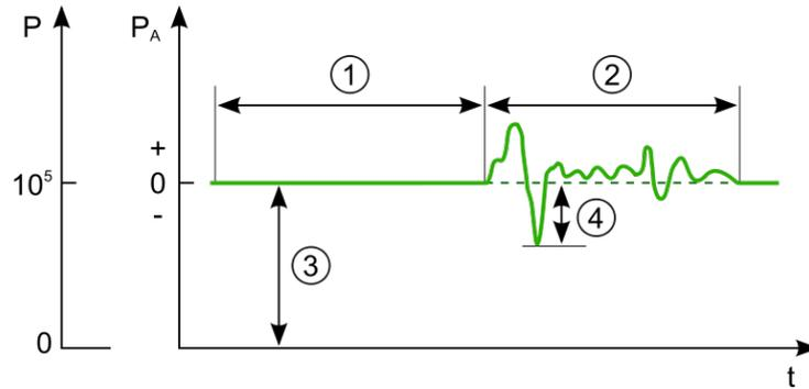
Figure 1.4: Sound pressure diagram: 1 – Silence, 2 – Audible sound, 3 – Atmospheric pressure, 4 – Instantaneous sound pressure
