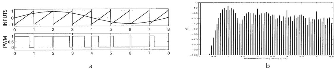
Figure 2.13: Natural sampling implementation: a – Time behavior, b – Frequency behavior
