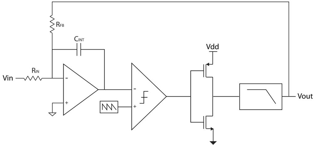
Figure 2.20: Single-ended closed-loop Class-D amplifier implementation
