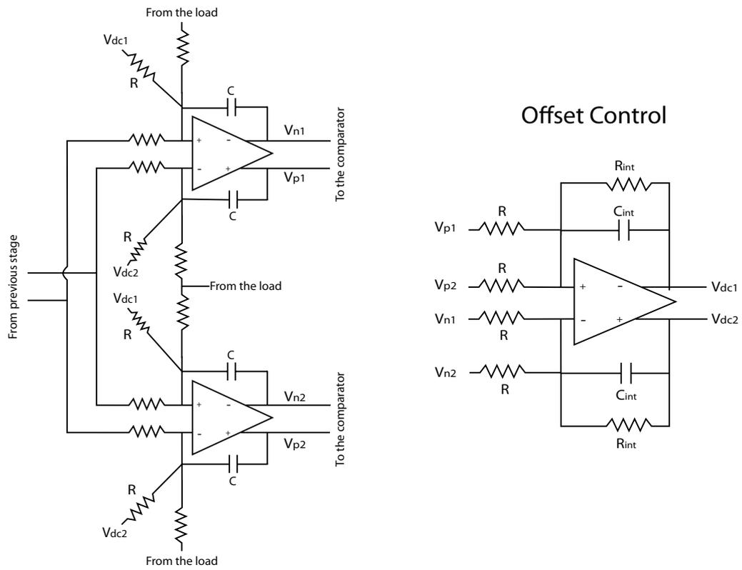
Figure 3.8: Carrier offset control circuit schematic
