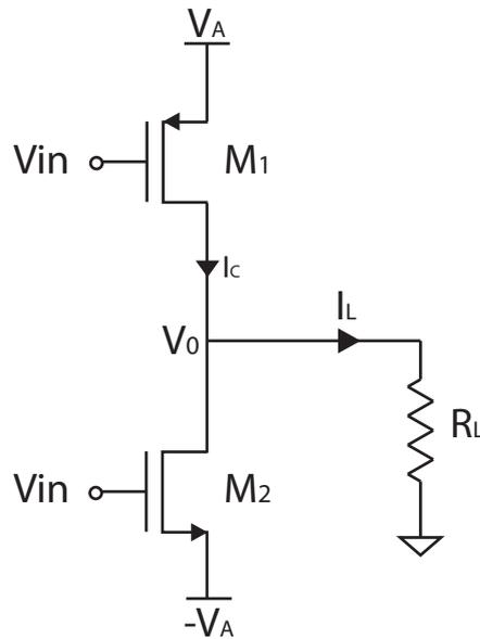
Figure 2.4: General Class-B schematic
