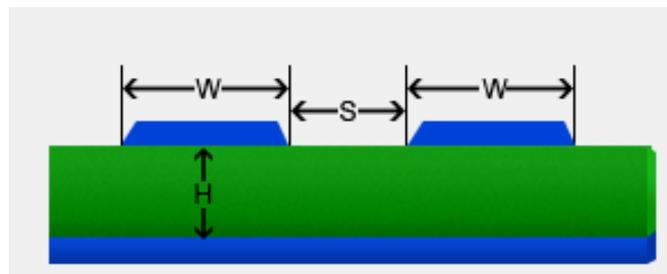
Figure 3.24: cross section of the microstrip.
