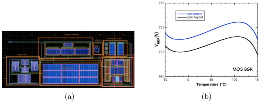
Figure 2.25: (a) layout and (b) comparison between pre and post layout simulations for the bandgap based on MOS devices
