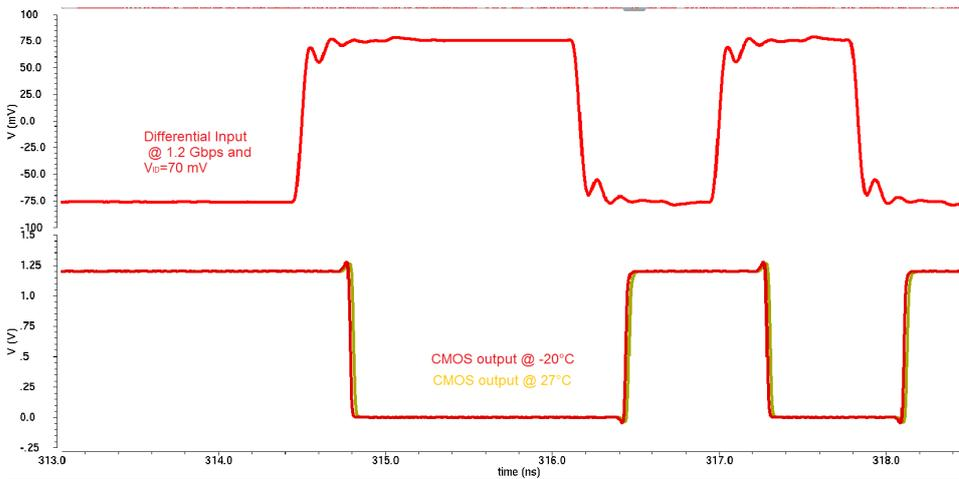
Figure 3.38: output CMOS of the receiver in worst case operating conditions ( $V_{ID} = \pm 70$  mV).
