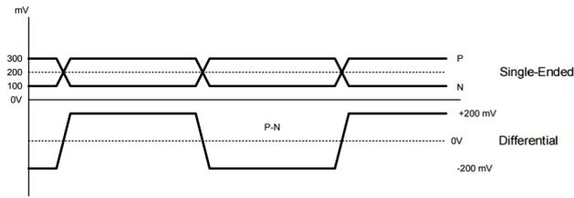
Figure 3.3: single ended and differential SLVS waveforms
