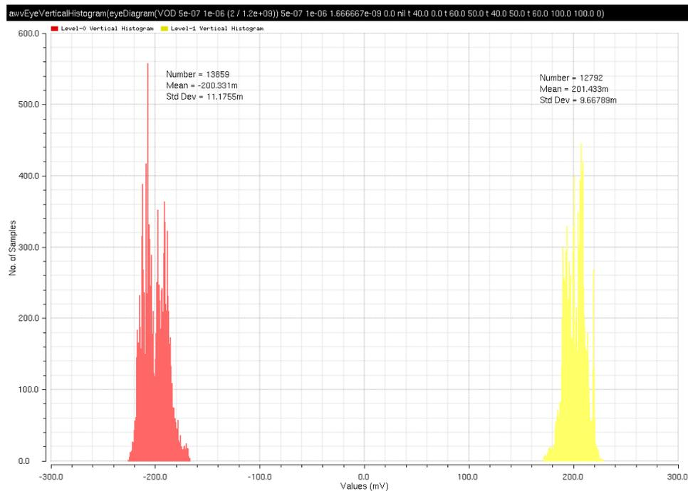
Figure 3.28: histogram of the eye diagram levels
