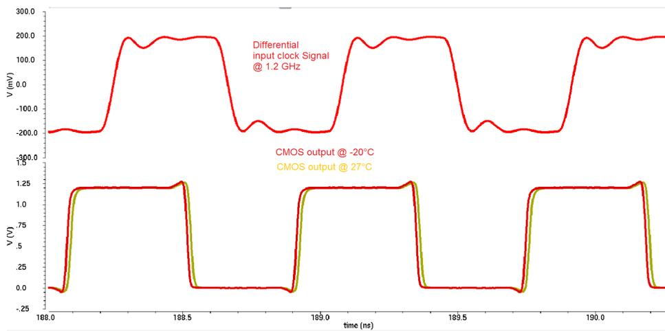
Figure 3.40: transient response of the receiver when a 1.2 GHz clock signal is applied for two operating temperatures:  $-20$  °C (red line) and  $27$  °C (yellow line).
