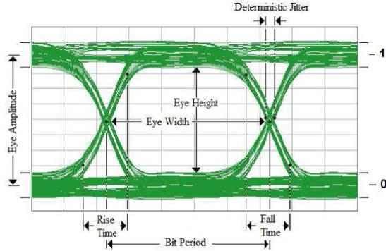
Figure 3.17: example of eye diagram with the relevant eye parameters.
