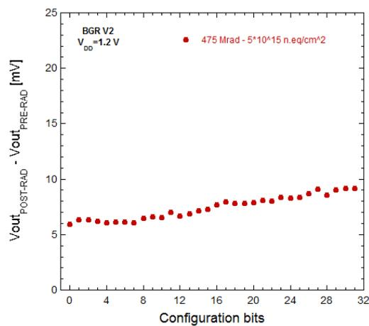
Figure 2.41: variation of bandgap output voltage after irradiation with 3 MeV protons at the CN accelerator in Legnaro.
