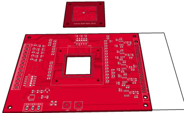
Figure 2.34: layout of the PCB test board.
