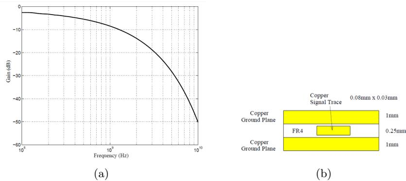
Figure 3.5: (a) S21 parameter and (b) cross-sectional view of 50  $\Omega$  (FR4) PCB stripline.
