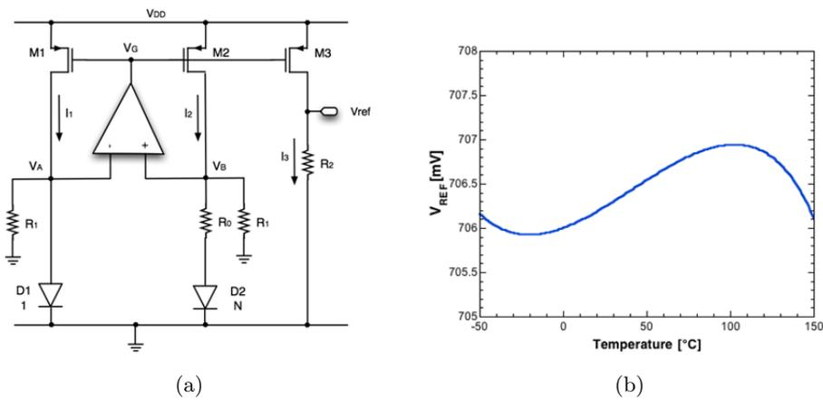
Figure 2.20: (a) schematic and (b) output voltage as a function of the temperature in nominal conditions for the bandgap reference circuit based on diode devices.
