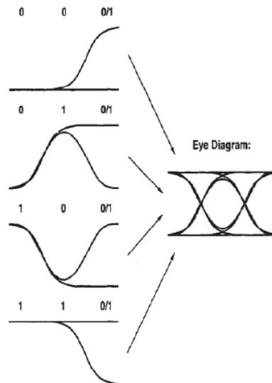
Figure 3.16: generation of the eye diagram.
