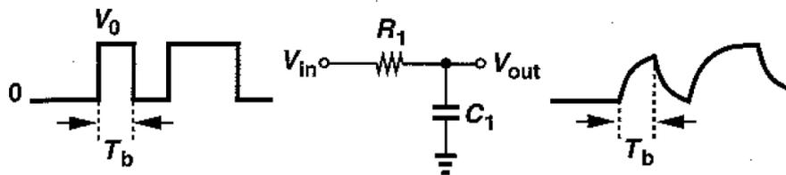
Figure 3.10: response of a single pole system to a random stream.
