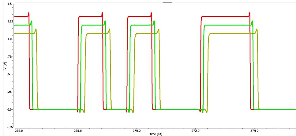
Figure 3.41: CMOS output of the receiver from PVT simulations. Red line refers to the fast corner, green line to the typical corner and yellow line to the slow corner.
