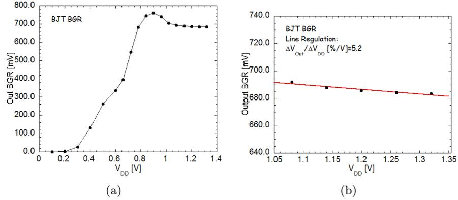
Figure 2.28: (a) output voltage of the bandgap vs power supply and (b) line regulation for the bandgap based on bipolar devices.
