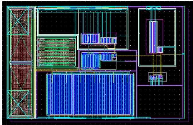
Figure 3.44: layout of the SLVS receiver.
