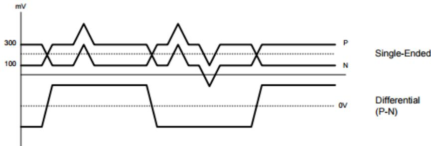
Figure 3.4: common-mode noise rejection.
