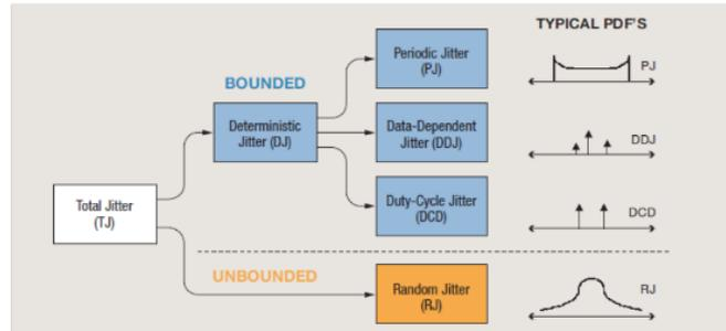
Figure 3.14: main components of the jitter: noise, system-phenomena and data-dependent contributions.
