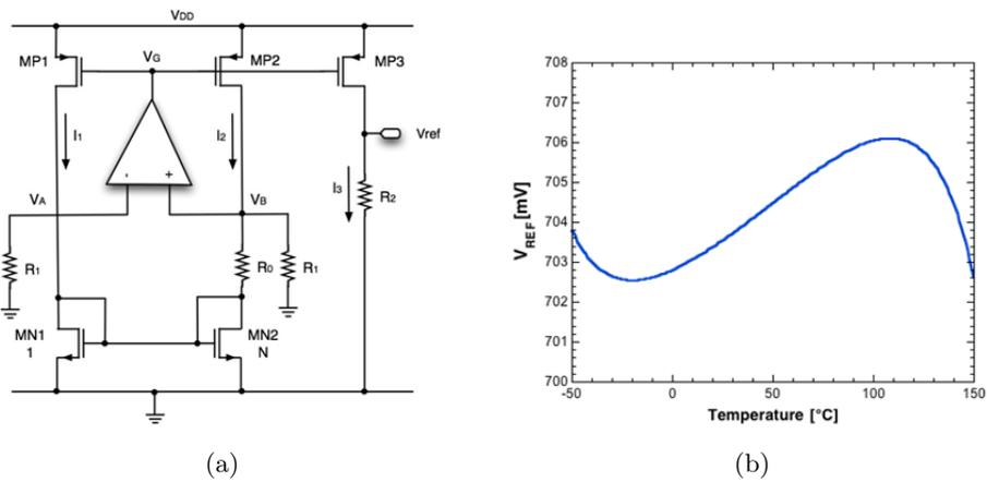
Figure 2.23: (a) schematic of the bandgap based on MOS in sub-threshold region and (b) output voltage as a function of the temperature in nominal conditions.
