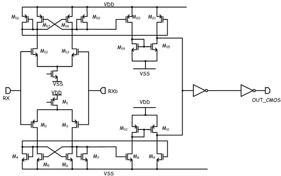
Figure 3.34: schematic of the receiver.
