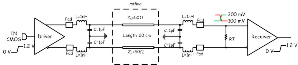
Figure 3.23: test bench for the transmitter.
