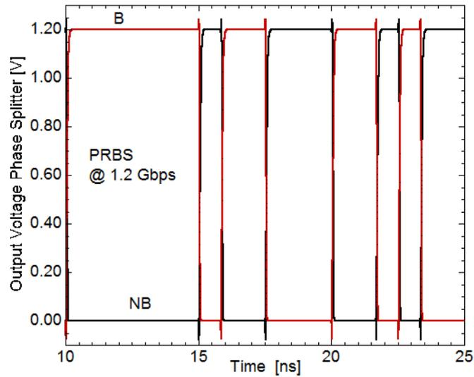
Figure 3.21: outputs of the Phase Splitter block, when at the input a PRBS signal at 1.2 Gbit/s is applied.
