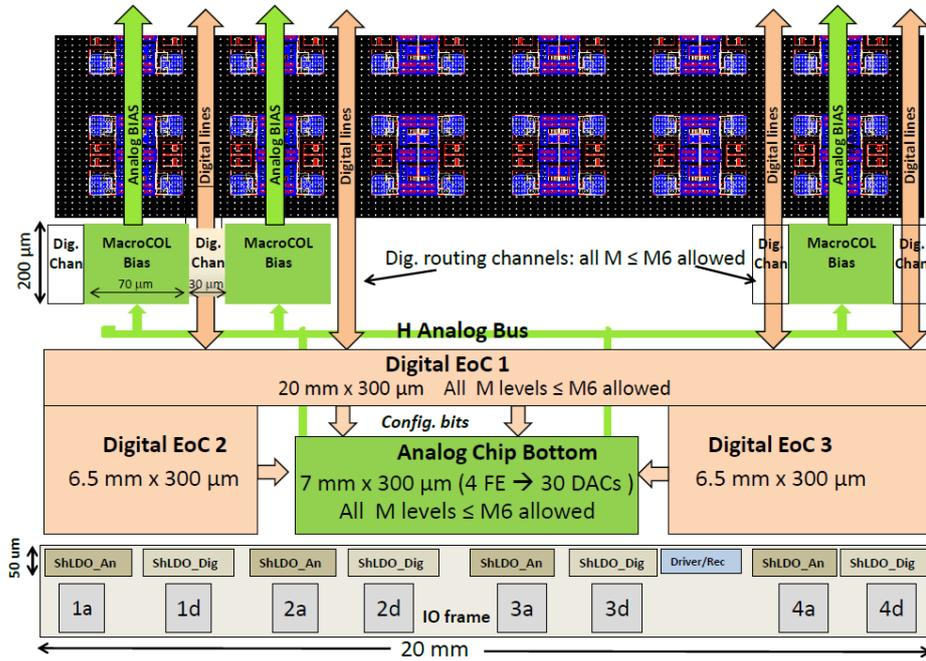
Figure 1.9: preliminary floorplan of the RD53A chip
