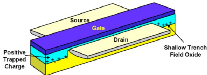
Figure 2.3: conceptual drawing (not to scale) showing how positive charge build-up in STI oxides can lead to lateral leakage currents in NMOS devices.
