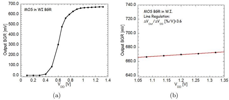
Figure 2.32: (a) output voltage vs power supply and (b) line regulation for the bandgap based on MOS transistors.
