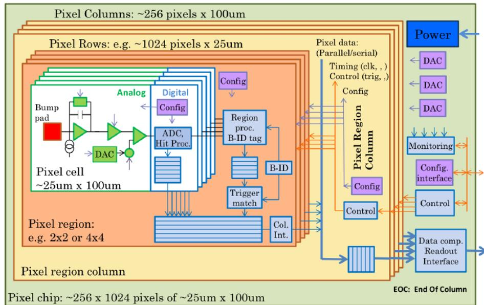
Figure 1.8: block diagram of the 3<sup>rd</sup> generation of front-end chip for the innermost layer of the CMS silicon tracker.
