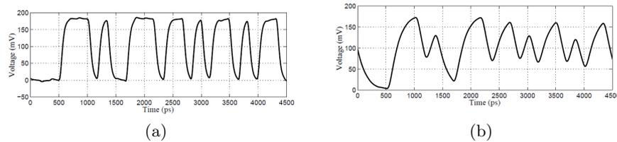
Figure 3.6: (a) data transmitted at 6 Gbit/s and (b) received signal at 6 Gbit/s affected by ISI due to a lossy channel.
