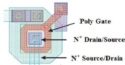
Figure 2.6: layout of an enclosed transistor (ELT) for rad-hard design.
