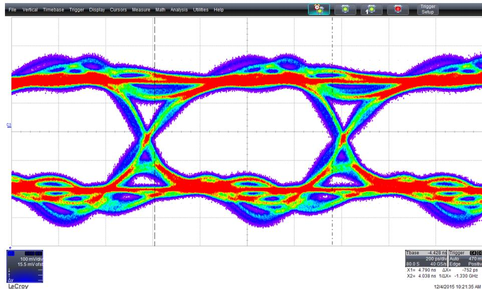
Figure 3.48: eye diagram at 1.2 Gbit/s of the transmitter signal.
