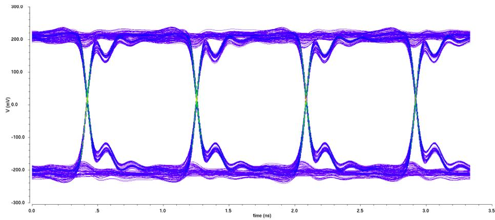
Figure 3.27: simulation of the transmitter eye diagram taken at the input termination resistance of the receiver.
