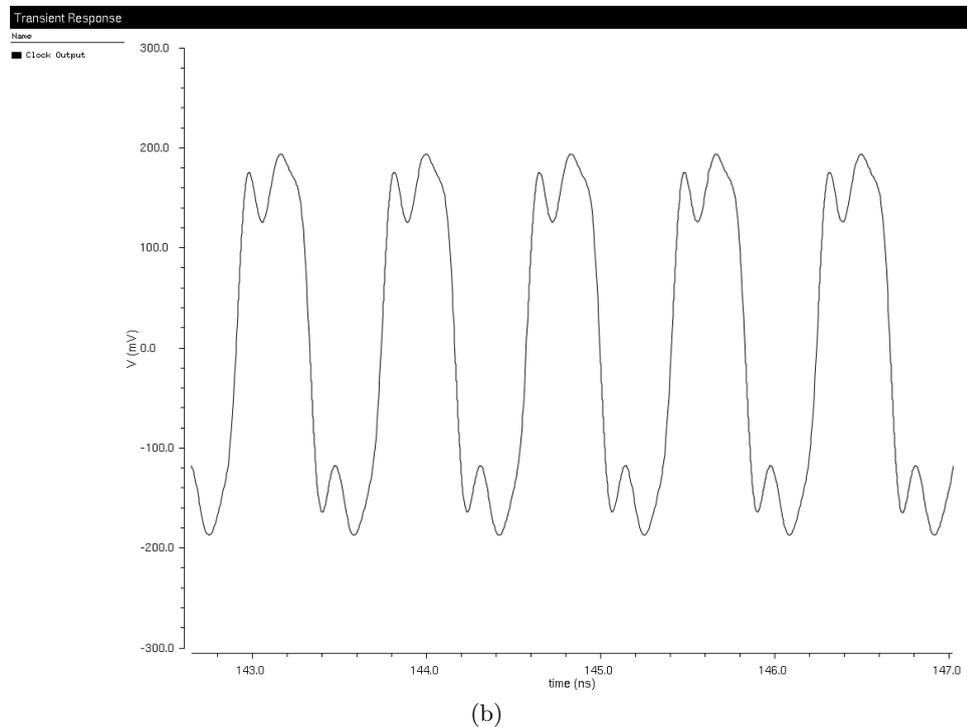
Figure 3.29: (a) eye diagram of the transmitter output at  $-20\text{ }^{\circ}\text{C}$  and (b) transient response applying a clock input signal at  $-20\text{ }^{\circ}\text{C}$ .
