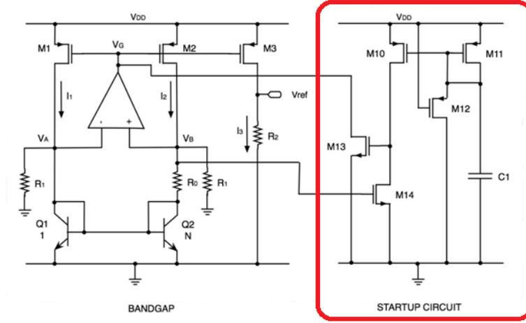
Figure 2.15: schematic of the proposed startup circuit.
