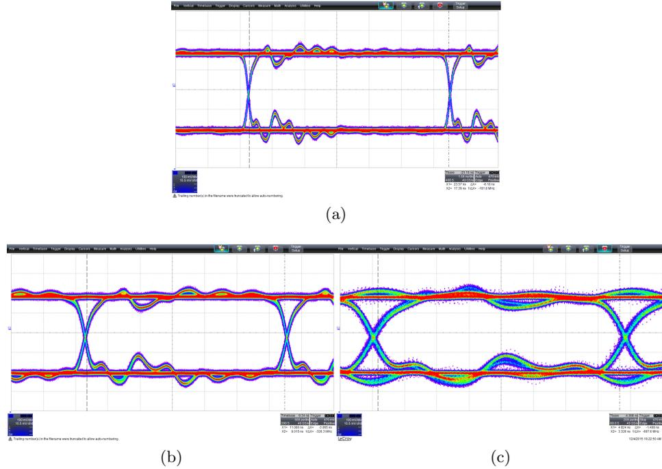
Figure 3.50: measurements of the eye diagram of the transmitter at (a) 160 Mbit/s, (b) 320 Mbit/s and (c) 640 Mbit/s.
