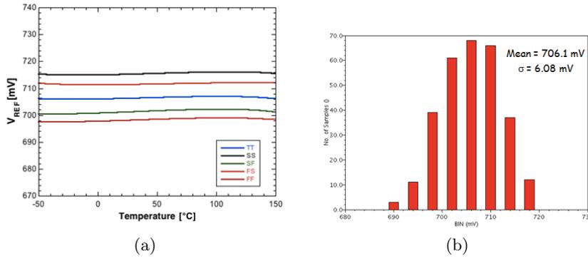
Figure 2.21: (a) output voltage as a function of the temperature as obtained from four corners simulations and (b) Monte Carlo simulation results for the bandgap based on diodes.
