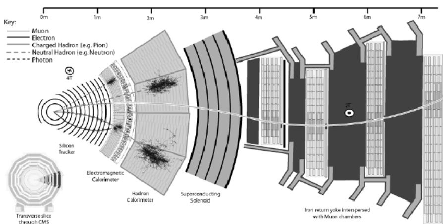
Figure 1.3: transverse section of the CMS detector and signatures for different particles crossing the volume.
