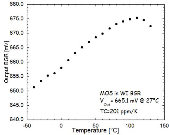
Figure 2.31: output voltage vs. temperature for the bandgap based on MOS devices in weak inversion.
