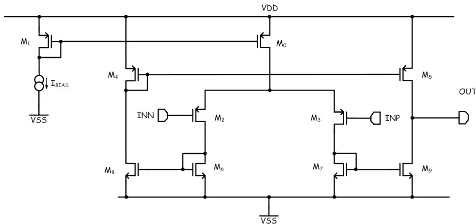
Figure 3.19: schematic of the symmetrical operational amplifier
