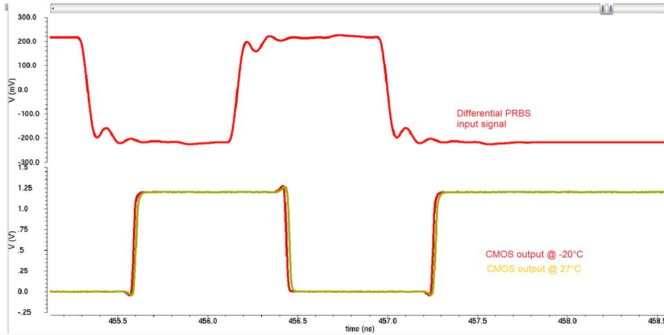
Figure 3.37: top plot is the PRBS differential input of the receiver at 1.2 Gbit/s and peak value  $V_{ID} = \pm 200$  mV. The bottom plot is the transient response of the receiver in nominal conditions for two different temperatures,  $-20^\circ\text{C}$  (red line) and  $27^\circ\text{C}$  (yellow line).
