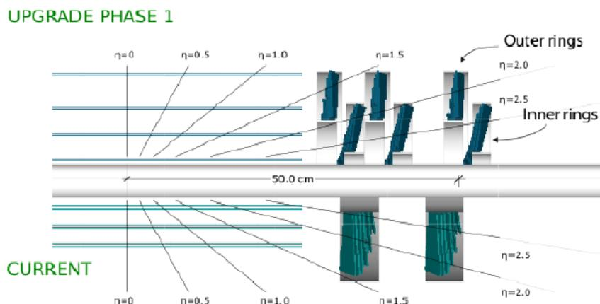
Figure 1.6: comparison between the current 3 layers (bottom) and the *Phase 1 upgrade* 4 layers for the CMS silicon tracker.
