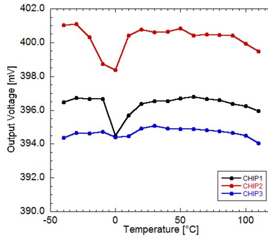
Figure 2.38: bandgap output voltage as a function of the temperature for three different chips.
