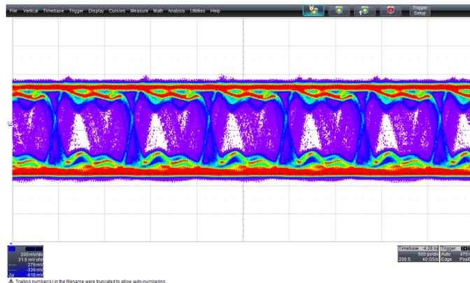
Figure 3.53: eye diagram of the receiver, as a response to a differential PRBS at 1.2 Gbit/s and differential input of  $V_{ID} = 100$  mV (worst case condition). The measurement has been performed at the output of the CML driver.
