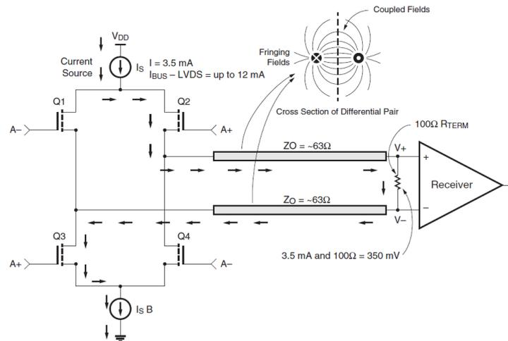
Figure 3.1: point-to-point LVDS link.
