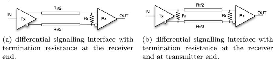
Figure 3.2: differential solution for high-speed data link.
