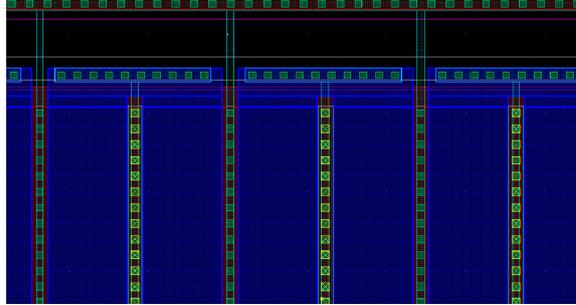
Figure 2.7: example of an enclosed layout for a multifinger device.
