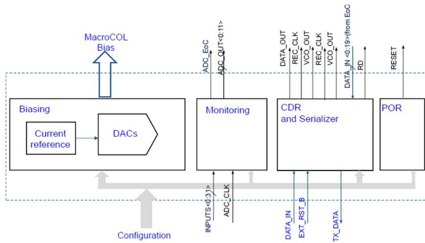
Figure 1.15: analog chip bottom block diagram.
