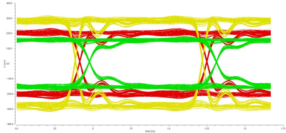
Figure 3.31: eye diagram simulated in three different corners: the green diagram obtained in the slow corner, the red one in the typical corner and the yellow one in the fast corner.
