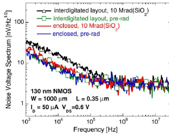
Figure 2.8: Noise voltage spectra before irradiation and after exposure to a 10 Mrad total dose for NMOSFETs with enclosed layout and with interdigitated layout, at 50  $\mu\text{A}$ .
