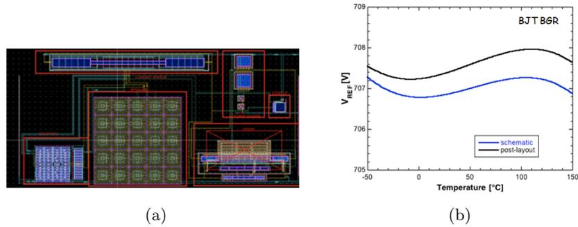
Figure 2.19: (a) proposed layout and (b) comparison between pre and post layout simulations of the bandgap reference with bipolar transistors.
