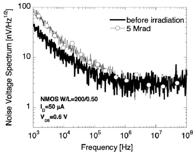
Figure 2.5: Noise voltage spectra before irradiation and after exposure to a 5 Mrad total dose of X-rays for an NMOS with W/L=200/0.5 in the 65 nm process, at 50 μA drain current.
