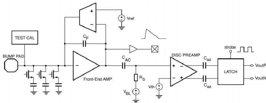
Figure 1.14: schematic of the analog pixel front-end designed at INFN Torino.
