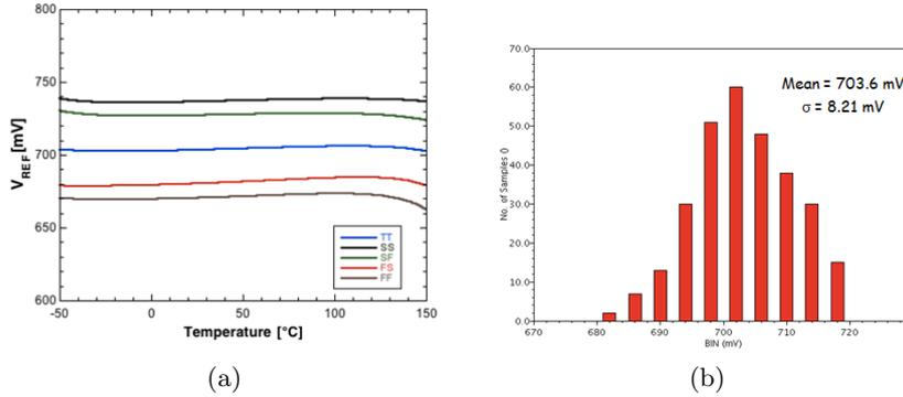
Figure 2.24: (a) output voltage for four corners simulations and (b) Monte Carlo simulations for the bandgap output voltage at room temperature.
