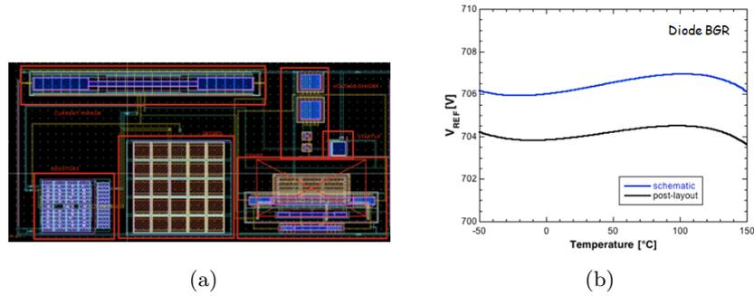
Figure 2.22: (a) layout and (b) comparison between pre and post layout simulations for the bandgap with diodes.
