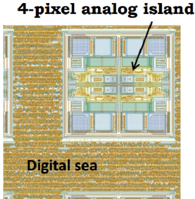
Figure 1.10: example of the new design approach. Four custom analog pixels are surrounded by a digital sea, where the digital standard cells are automatically placed and routed by synthesis tool.
