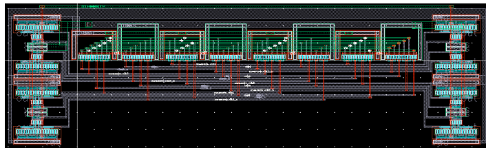
Fig. A.9 Switch box includes 32 switches for the implementation of the current spinning technique.
