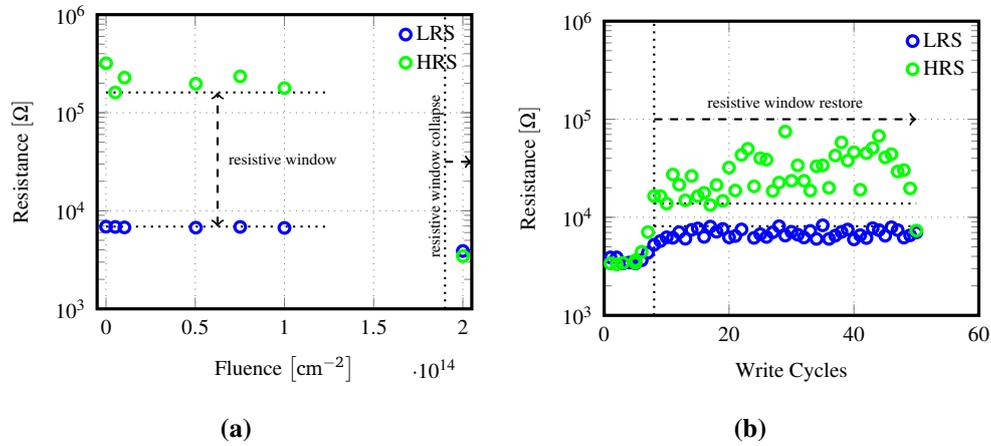
**Figure 4.14:** LRS/HRS state of a single 1T1R ReRAM cell for different 1.8 MeV proton fluences, [4.32]. The loss of the resistive windows occurs for fluences higher than  $2 \times 10^{14} \text{ cm}^{-2}$ .
