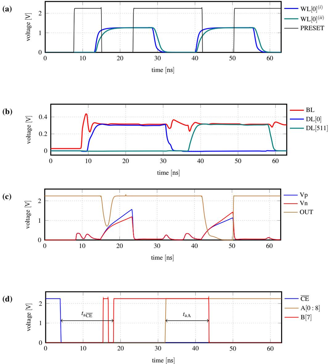
**Figure 6.28:** Simulation (worst case corner - wcc) of two read accesses. In the simulation two cells are accessed: first the cell at the beginning of the word-line is accessed (*i*), triggered by the *chip enable* signal ( $\overline{CE}$ ) asserted low; then the cell at the end of the word-line (*ii*) is accessed as soon as the address input word toggles.
