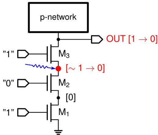
**Figure 5.5:** Example of erroneous switch due to a single event in a series connection of transistors.
