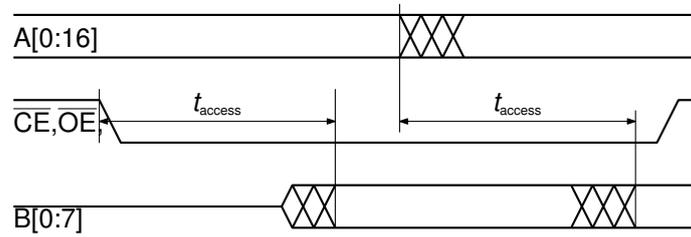
**Figure 6.8:** Simplified time diagram for an asynchronous read access. Data access is triggered by the transitions of control signals (OE and CE that are active low inputs) and addresses.
