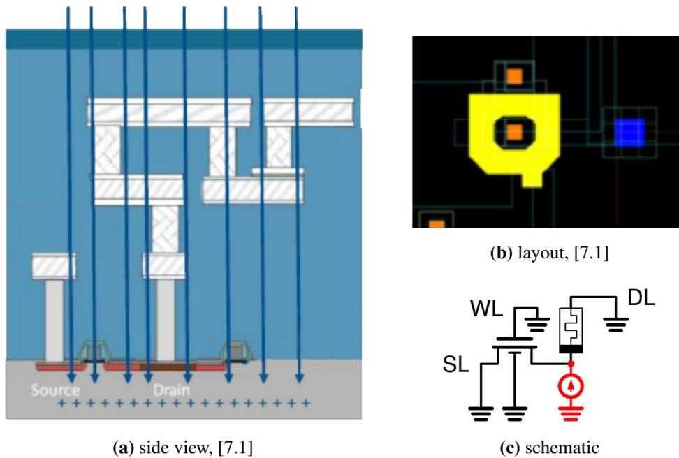
**Figure 7.13:** Representation of the high energy particle damage induced in the device.
