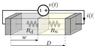
**Figure 4.6:** Representation of the model proposed by Strukov, [4.2]. The global resistance is the series of the doped and undoped layers' resistances.
