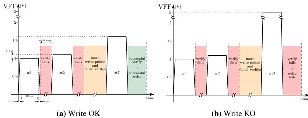
**Figure 6.6:** Time diagram of a *Write & Verify* operation.
