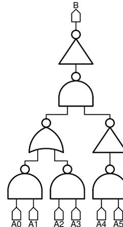
**Figure 5.6:** Example of a 6 input AND implementation by mean of two inputs basic gates.
