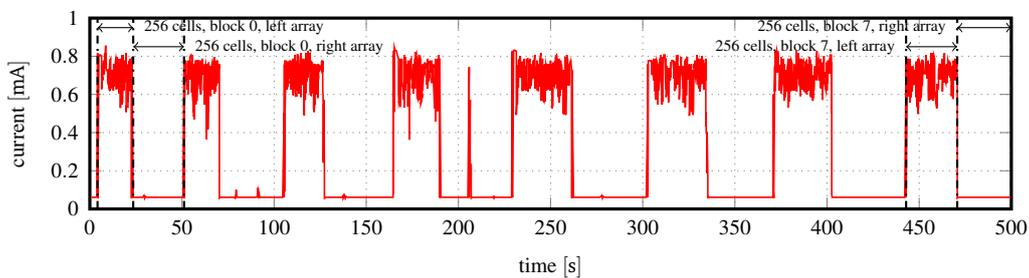
**Figure 7.20:** Example of a read scan of the resistive cells, [7.1]. All 8 blocks are scanned. Results refers to an exposure of 134.31 krad.
