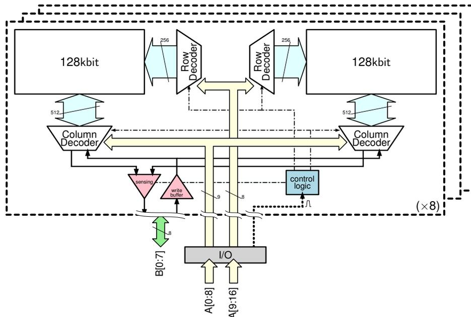
**Figure 6.14:** Functional scheme of the single block. The row decoder asserts the 512 memory cells; one of them, then, is connected by the column decoder, according to the operation to be carried out, either to the read-out circuits or to the write switches. Each block is also provided with its own control logic block.
