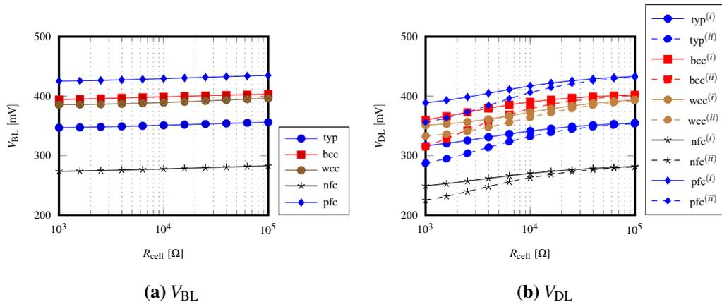
**Figure 6.25:** DC simulations of the regulated voltage, sweeping the resistance value ( $R_{\text{cell}} = 1 \div 100\text{k}\Omega$ ), over all the process corners. The bias used is the internal generated one. In (a) is plotted the voltage directly driven by the voltage regulator, while (b) are represented the voltage at the memory cell drain-line, for the near (i) and far (ii) cells.
