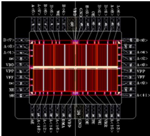
**Figure 7.1:** Bonding diagram of the 1 Mbit chip for a DIL 48 package.
