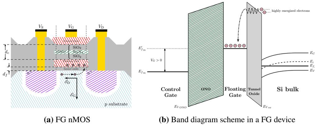
**Figure 3.3:** FG device. Structure and band diagrams.
