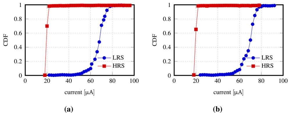
**Figure 7.12:** Post irradiation cycling: recovered CDFs of HRS and LRS states after irradiation with Xenon ions (a) and protons (b).
