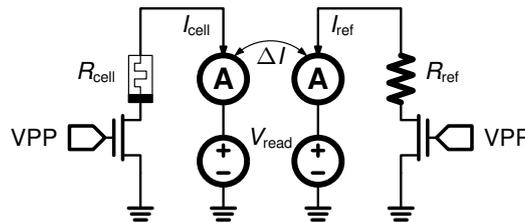
**Figure 6.10:** Digital read scheme for memristive memories. The resistance values are compared by mean of a current comparison.
