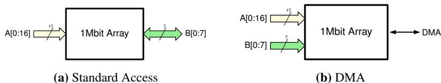
**Figure 6.7:** Access modes of the 128 kB ReRAM test device. For standard access mode (a) the B bus is used for the I/O, while in DMA mode (b) the B bus addresses one selected bit out of eight.
