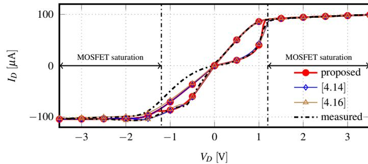
**Figure 4.8:** Measured I-V characteristics versus estimated values. The extracted parameters are:  $R_{\text{on}} = 7\text{ k}\Omega$ ,  $R_{\text{off}} = 60\text{ k}\Omega$ , and  $\tilde{K}_I = 4.50 \times 10^9 \Omega/\text{C}$ .
