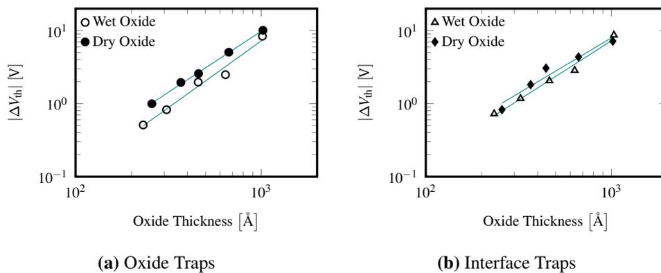
**Figure 2.8:** Dependency of radiation-induced threshold voltage shifts.
