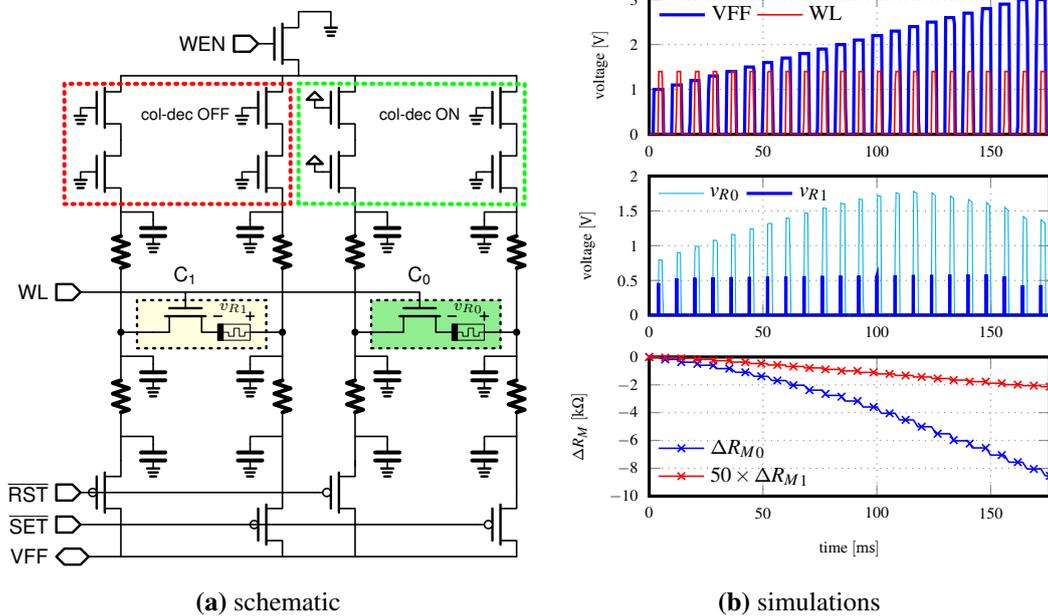
**Figure 6.21:** Simulations of a *set* operation for two 1T-1R cells connected to the same word-line. Cell 0 is accessed and written. If source-lines are precharged to ground, cell 1 is affected by a spurious *set* due to source-line charge.
