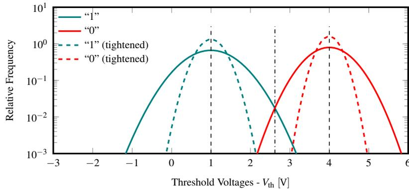
**Figure 3.5:** Threshold voltage distributions in a flash device.
