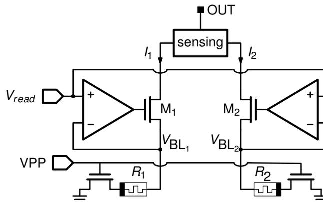
**Figure 6.22:** Reading principle scheme.
