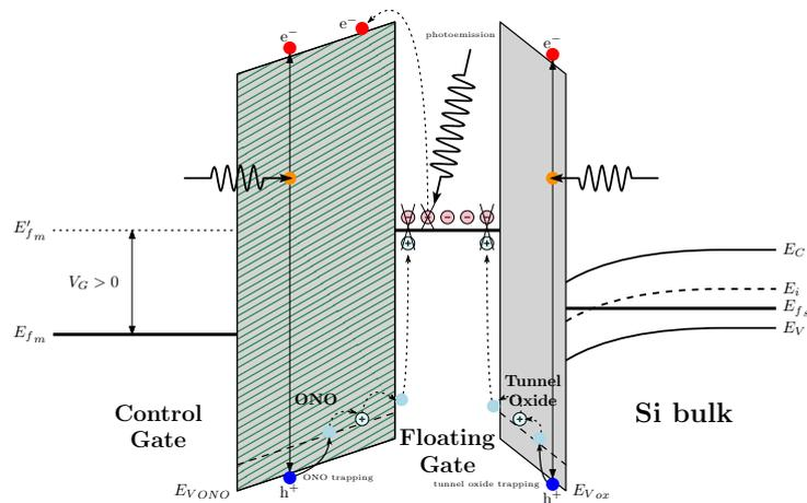
**Figure 3.6:** Scheme of the radiation-induced effects in a FG cell.
