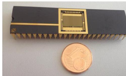
**Figure 7.2:** Demonstrator assembled into a DIL 48 package, [7.1].
