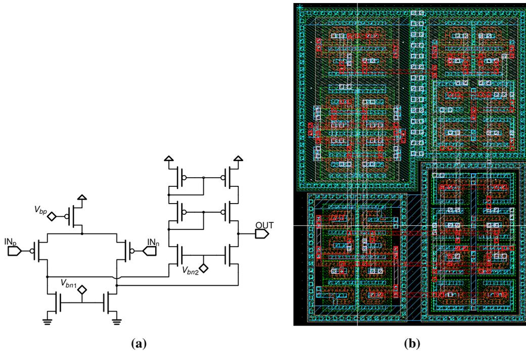
**Figure 6.30:** Schematic (a) and layout (b) of the folded cascode Operational Amplifier implemented with ELTs.
