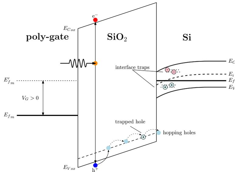
**Figure 2.3:** Band diagram of a MOS structure under the action of a direct gate voltage. The hopping movement of the holes is shown. During their drift holes are trapped by either oxide or interface traps.
