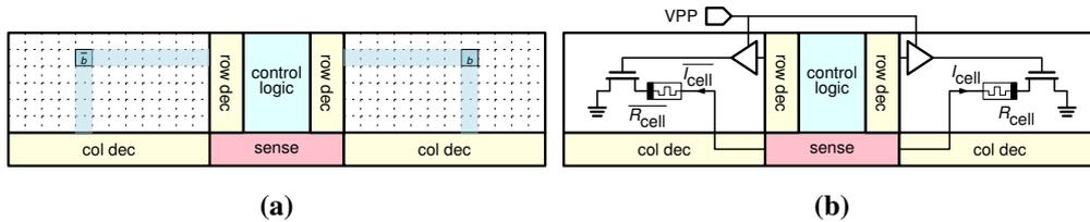
**Figure 6.12:** Differential approach. The memory array is split in two parts, whereas one single bit  $b$  is stored complementary in two symmetrical locations (a). When a data is accessed, the resistance values of the two symmetrical locations are compared (b).
