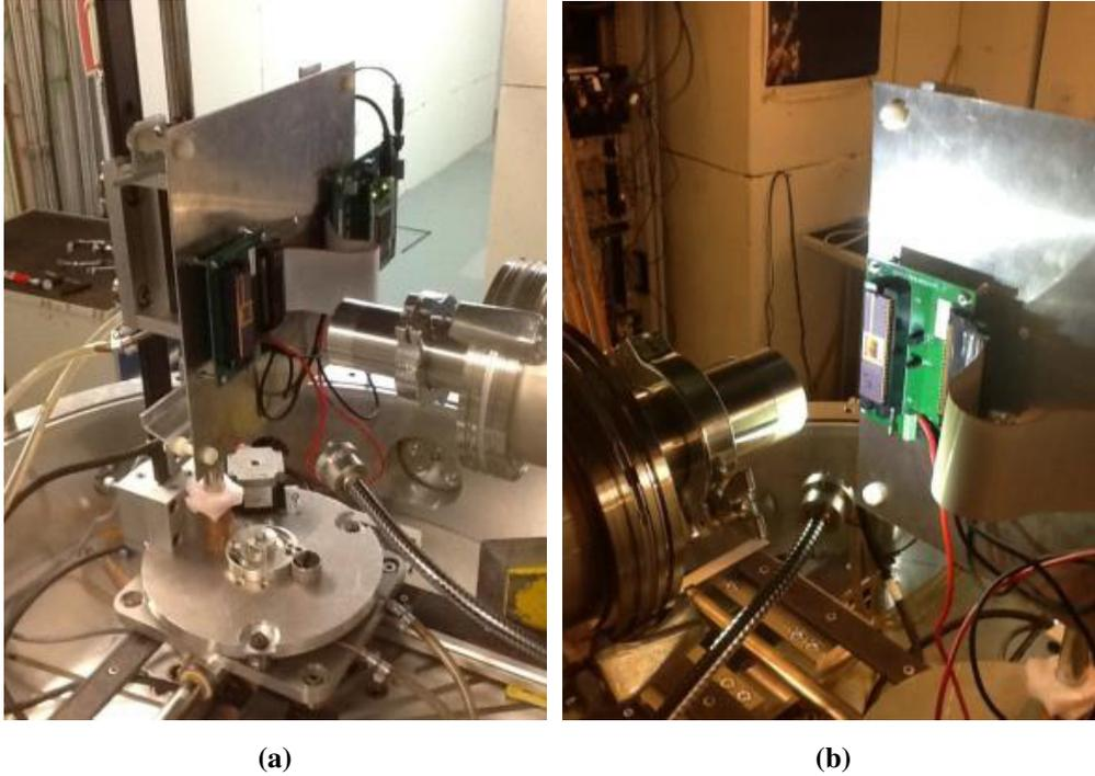
**Figure 7.6:** Board positioning for ion beam, [7.1].
