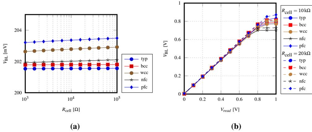
**Figure 6.26:** Simulation results of the regulated voltage  $V_{BL}$  over all the process corners, sweeping the resistance value  $R_{cell}$  for a  $V_{read} = 200\text{ mV}$  (a) and varying the external read voltage for  $R_{cell} = 10\text{ k}\Omega$  and  $R_{cell} = 20\text{ k}\Omega$  (b).
