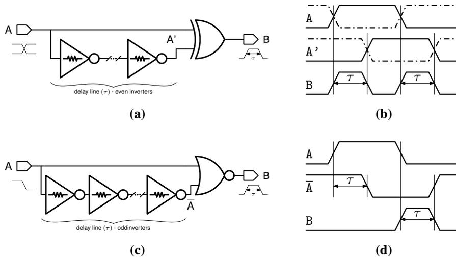
**Figure 6.9:** CMOS implementation for an ATD circuit (a) and a active-low control signal transition circuit (c). Respective time diagrams are (b) and (d).
