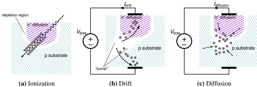
**Figure 2.14:** Charge collection mechanism in a single event. The radiation particle ionizes the substrate (a) generating free charge carriers that are drifted by the applied electric (b) and then neutralized by diffusion (c).
