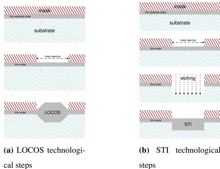
**Figure 2.10:** Substantial technological steps of the LOCOS and STI manufacturing.
