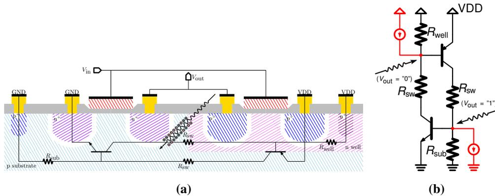
**Figure 2.16:** Scheme of a CMOS inverter implementation representing a scheme of the parasitic BJTs
