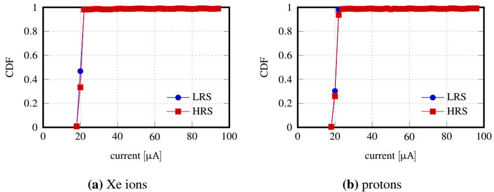
**Figure 7.11:** CDFs of HRS and LRS states after irradiation with Xenon ions (a) and protons (b).
