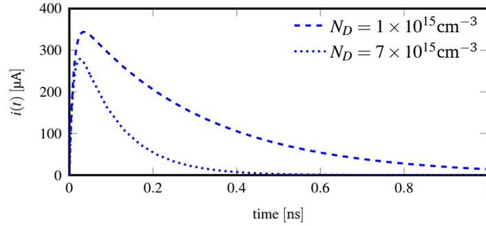
**Figure 2.15:** Transient response for a 5 MeV  $\alpha$ -particle with different doping concentrations, [2.22].
