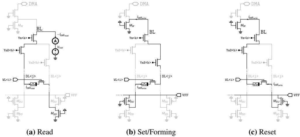
**Figure 6.19:** Standard access examples for *read* (a), *set* (b) and *reset* (c) operations. In (a) the column decoder connects the selected cell to the read circuits and the read current has a path to ground thanks to the switch transistor  $M_{SD}$ . In (b) and (c), VFF drives all the columns through the switch transistors  $M_{DU}$  ( $M_{SU}$ ), but only the selected one has a current path to ground through the final stage of the column decoder, thanks to the transistor  $M_W$ .
