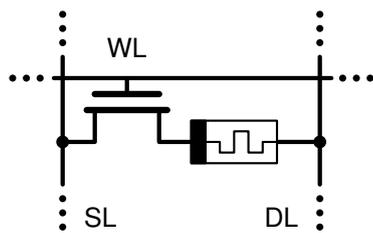
**Figure 6.2:** Schematic of the 1T1R cell.
