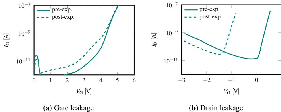
**Figure 2.9:** Radiation-induced leakage currents before and after irradiation of a n-channel MOS device. In (a) the gate current before and after irradiation of a n-channel MOS device exposed to 5.3Mrad of  $^{60}\text{Co}$   $\gamma$ -rays, while in (b) the drain current before and after irradiation of a n-channel MOS device exposed to 1Mrad of  $^{60}\text{Co}$   $\gamma$ -rays.
