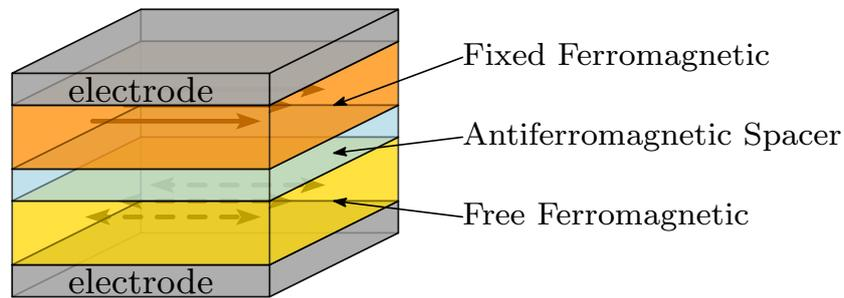
**Figure 4.2:** Scheme of a magnetoresistive device element.
