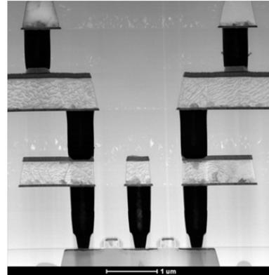
**Figure 6.4:** TEM image of two 1T-1R cells, sharing the source-contact. The resistive MIM cells are placed on metal 2.
