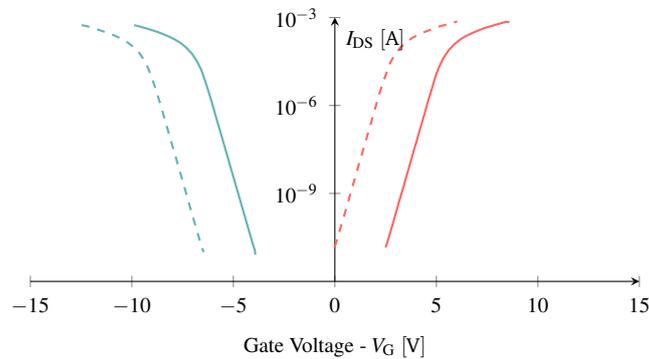
**Figure 2.6:** Representation of the threshold voltage shift for both a nMOS and a pMOS.
