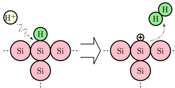
**Figure 2.5:** Interface trapping mechanism. Protons capture hydrogen electrons and form a new  $\text{H}_2$  molecule.
