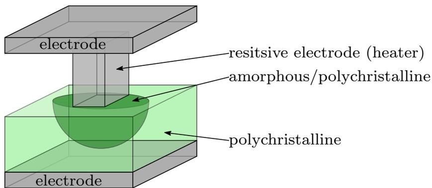
**Figure 4.3:** Scheme of a phase-change device element.
