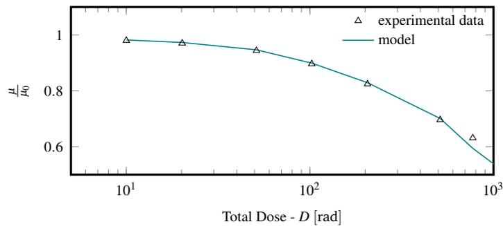
**Figure 2.13:** Experimental and modeled mobility damage versus the total ionizing dose  $D$ , [2.17].
