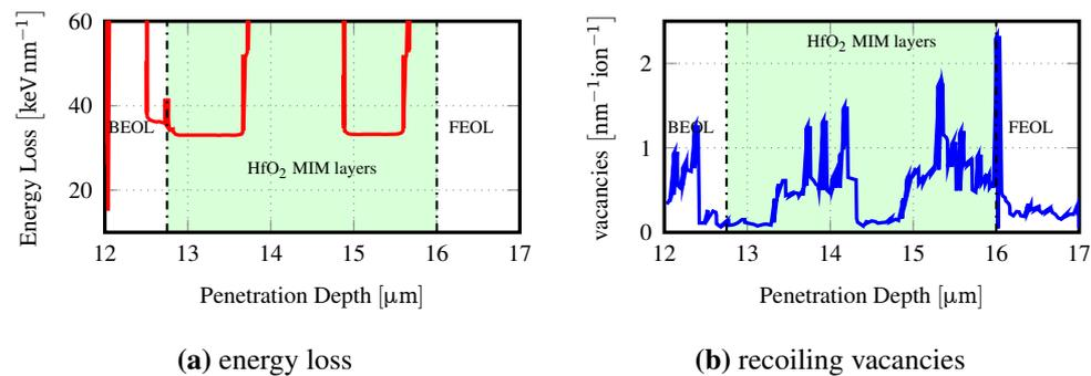
**Figure 7.15:** SRIM estimations for Xenon ions. Zoom of the HfO<sub>2</sub> layer.
