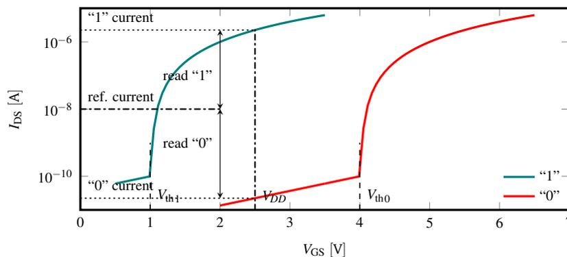
**Figure 3.4:** Currents in a FG device and reading principle. When a FG cell is selected, the relative current is compared with a reference and the digital value discriminated.
