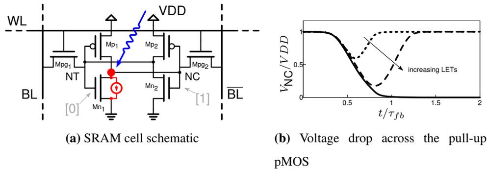
**Figure 3.2:** SEU mechanism in a SRAM cell.
