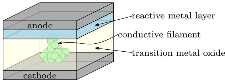
**Figure 4.4:** Scheme of the MIM stack of the resistive device.
