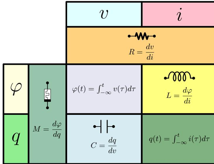
**Figure 4.1:** Scheme of the Maxwell's equations for condensed parameters.
