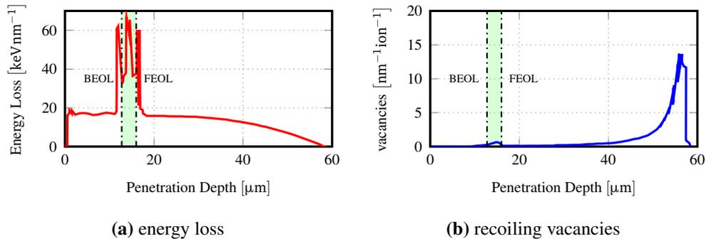
**Figure 7.14:** SRIM estimated energy loss and vacancies recoils for Xenon ions within the memory device.
