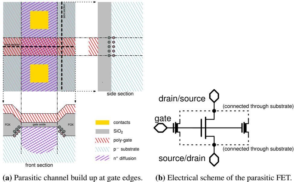
**Figure 2.11:** Description of the parasitic FET effect at the gate edges. The gate overlaps on the thin/thick interface create two built-in depleted field effect transistors (FETs).
