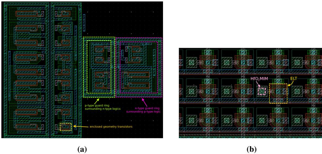
**Figure 6.29:** Layout examples. (a) Detail of the row-decoder: a 6-inputs NAND is shown. Guard rings and ELT are highlighted. (b) Detail of the memory array. ELT selectors and HfO<sub>2</sub> MIM are recognizable.
