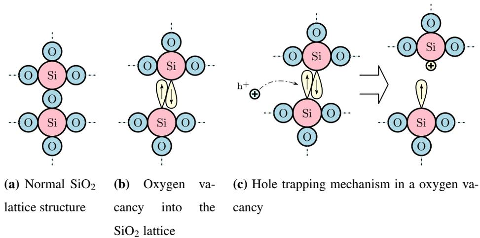
**Figure 2.4:** Oxide trapping mechanism. The radiation-generated hole accepts an electron made displaceable by an oxygen vacancy in the silicon oxide.
