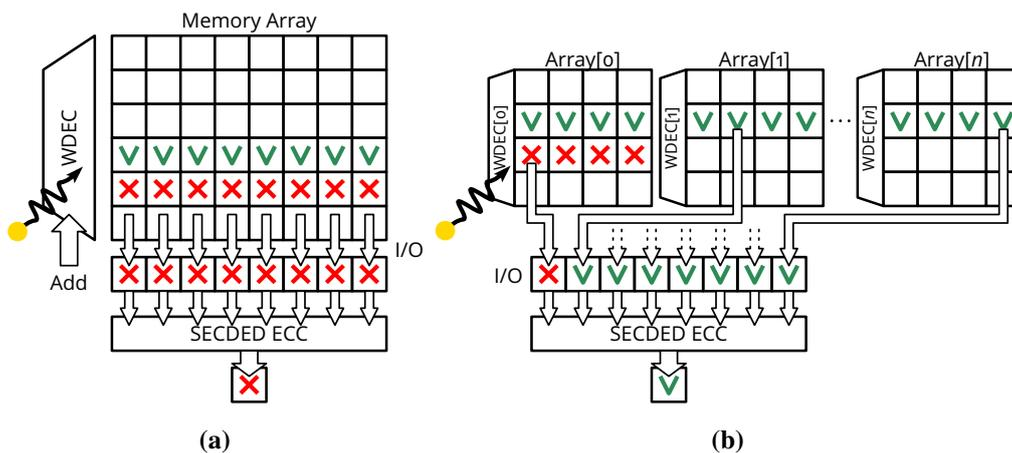
**Figure 5.7:** Single (a) and independent (b) memory array architectures.
