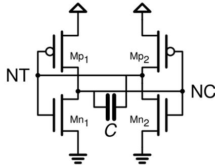
**Figure 5.4:** Cross coupled inverter pair with Miller Capacitor.
