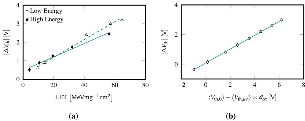
**Figure 3.8:** Threshold voltage dependence on LET incident energy (a) and electric field (b).
