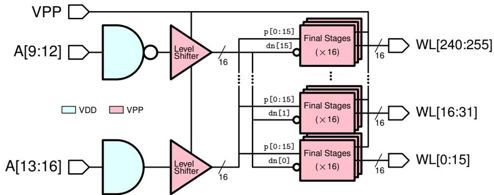
**Figure 6.15:** Row decoder scheme. A two level decoding has been implemented. Different colors have been used for different voltage domains.
