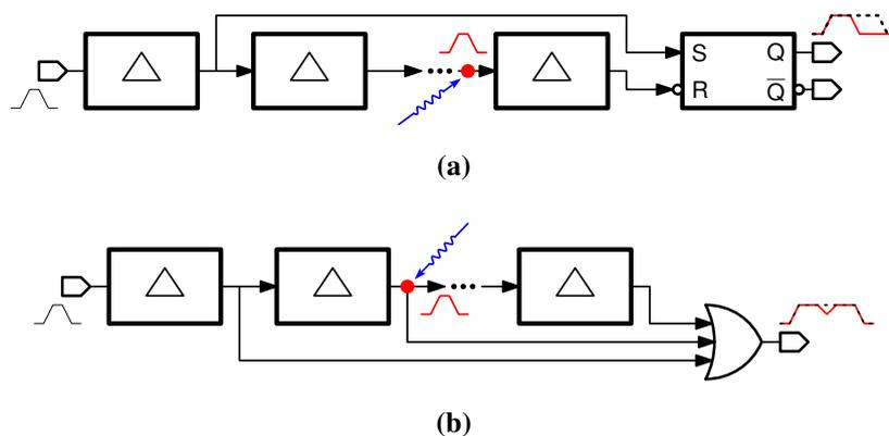
**Figure 5.8:** Different implementations of a digital phase.
