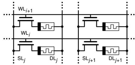
**Figure 4.12:** 1T-1R cell schematic.
