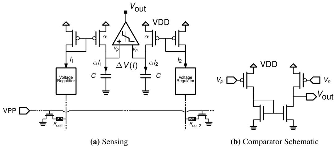
**Figure 6.27:** Sense amplifier schematic. Cell currents sunk by the voltage regulators are amplified by a current mirror, converted into a voltage ramp by capacitors and then compared.
