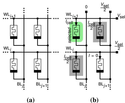
**Figure 4.10:** Sample of a crossbar array (a) and selection approach (b). Sneak current effects are also shown.
