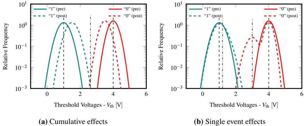
**Figure 3.7:** Radiation-induced threshold voltage shifts.
