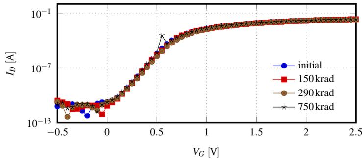
**Figure 7.19:** Before and after irradiation I-V characteristics of the 1T-1R cell ELTs, [7.1].
