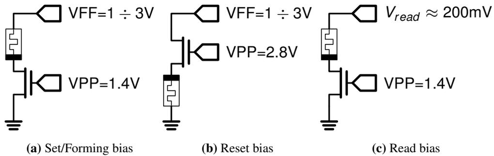
**Figure 6.5:** Biasing conditions for the bipolar cell operations. VFF is the Forming/Set/Reset voltage that has to be applied to the memristor, while the voltage VPP controls the compliance current in the different operations.
