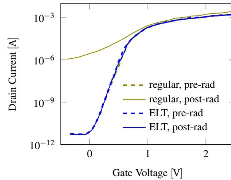
**Figure 5.2:** Pre- and post- irradiation experimental curves for edge-less and regular transistors.
