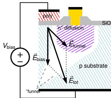
**Figure 2.17:** Scheme of a SEGR generation. The electric field across the funnel depletion volume  $E_{\text{funnel}}$  is added to the bias electric field  $E_{\text{bias}}$ , resulting in a higher electric  $E_{\text{tot}}$  across the gate oxide.
