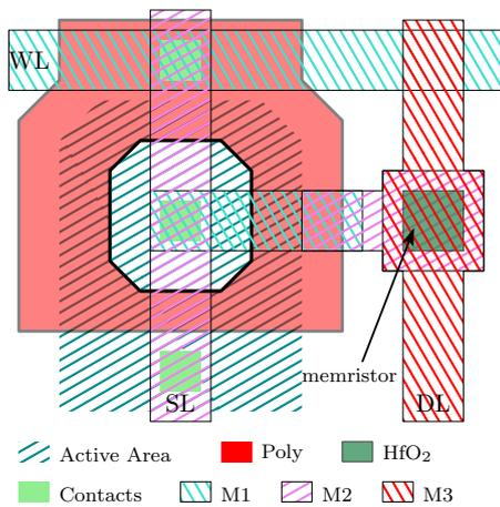
**Figure 6.3:** Scheme of 1T1R Cell layout implementation using an ELT. The memristive layer is sandwiched between metal 2 and metal 3.
