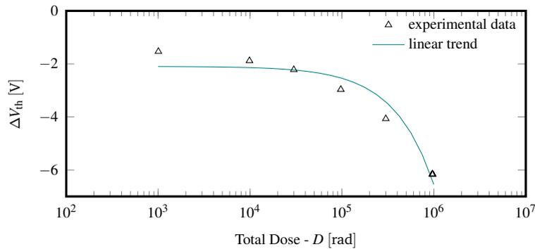
**Figure 2.7:** Threshold voltage shift versus total ionizing dose. The linear dependency on the total dose  $D$  can be recognized.
