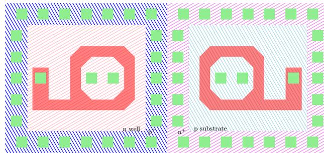
**Figure 5.3:** Example of layout implementing double guard rings.
