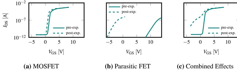
**Figure 2.12:** Measured data for leakage currents in the parasitic edge device.
