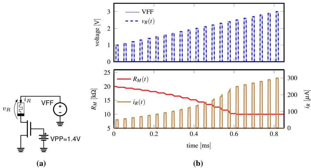
**Figure 4.9:** Simulation of a cell *set*. A pulse sequence is applied to the drain-line, while the transistor gate is driven with a DC voltage of 1.4 V. It is possible to notice the linear decrease of the resistance value when the voltage pulse is applied.
