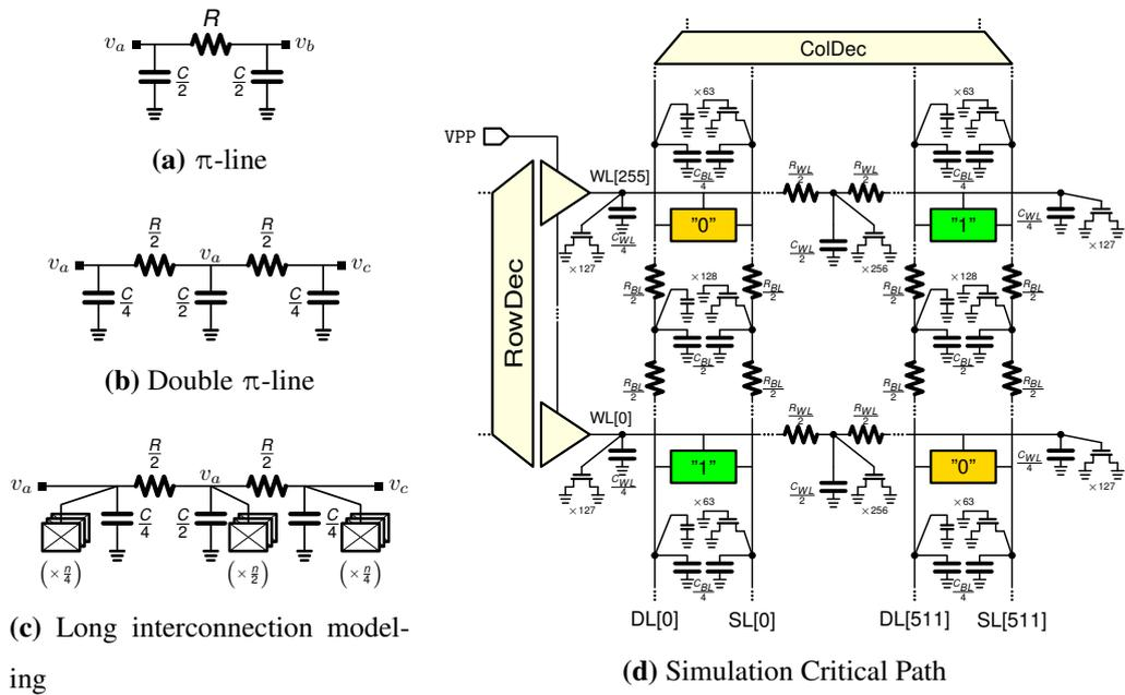
**Figure 6.1:** Simulation setup. (a) , (b) Modeling of a long metal interconnection having total resistance  $R$  and total capacitance  $C$  by mean of  $\pi$  transmission lines. (c) Long metal interconnection modeled by two  $\pi$  transmission lines with the contribution of  $n$  (capacitive) dummy loads. (d) Critical-Path circuit used for the simulations
