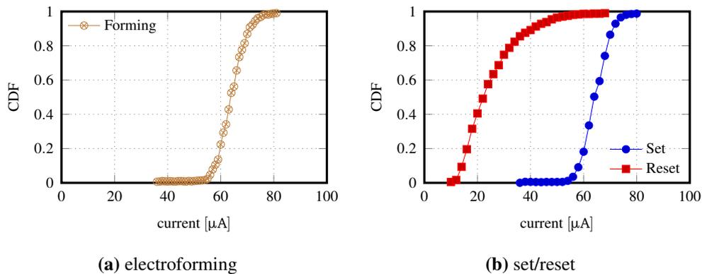
**Figure 7.10:** CDF of forming and HRS/LRS currents (after the first set and reset process).
