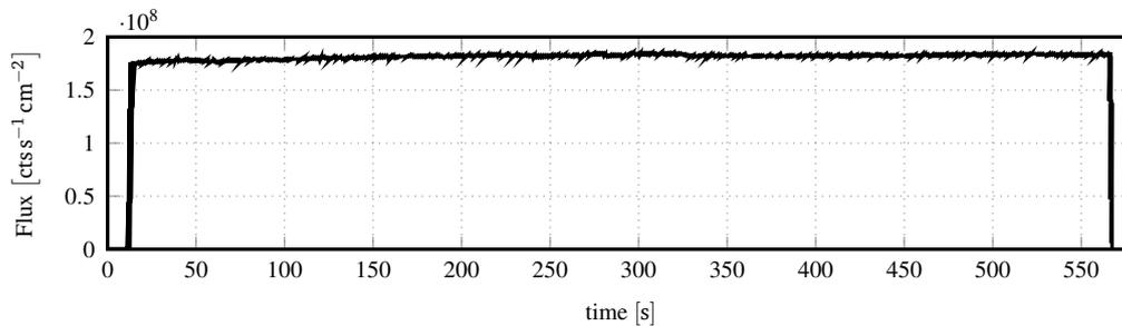
**Figure 7.9:** Example of proton flux during a test cycle, [7.1].
