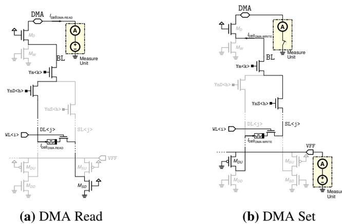
**Figure 6.20:** DMA examples for *read* (a) and write (*set*) (b). While read mode the measure unit (MU) can directly force the read voltage to the DMA pin, analogously to the standard mode, in the write configuration the MU should connect the DMA pin to ground.
