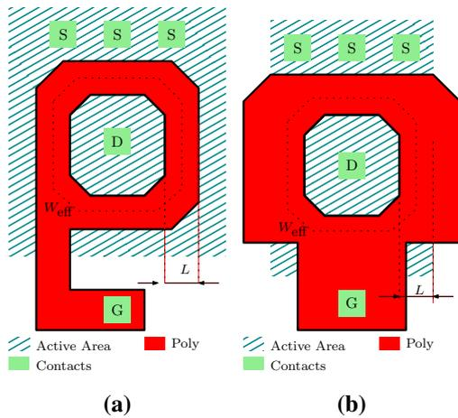
**Figure 5.1:** Examples of enclosed gate geometries. The geometry in (a) has a larger drain area, while the one in (b) offers a larger gate area and a smaller drain area.
