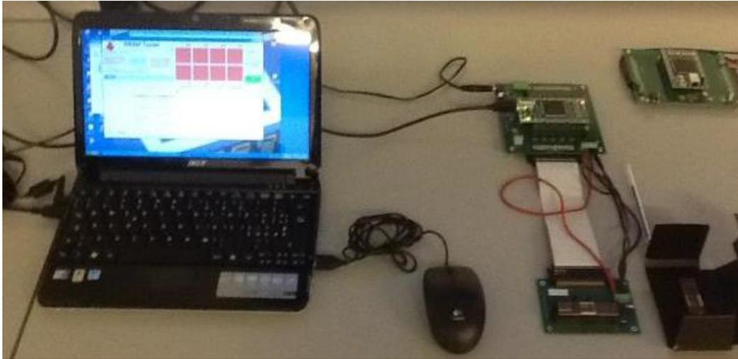
**Figure 7.5:** Setup board connection via USB to laptop PC, [7.1].
