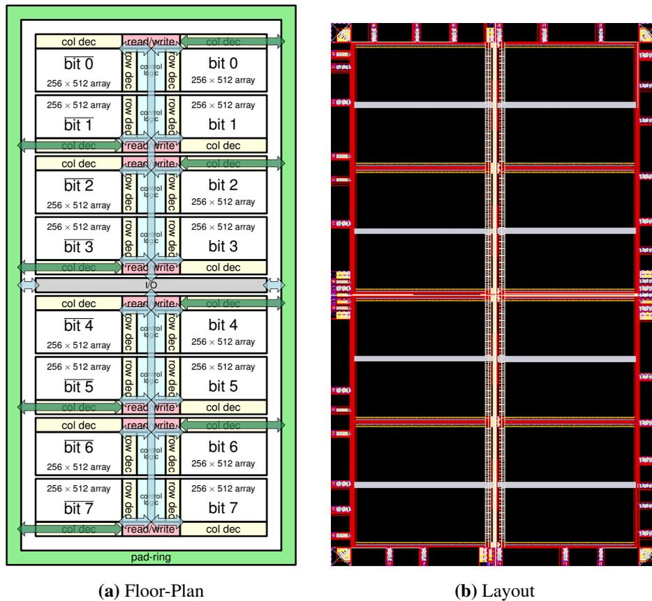
**Figure 6.13:** Floor-plan (a) and layout (b) of the 1 Mbit memory device. The whole array is split among 8 independent blocks of 128 kbit each.
