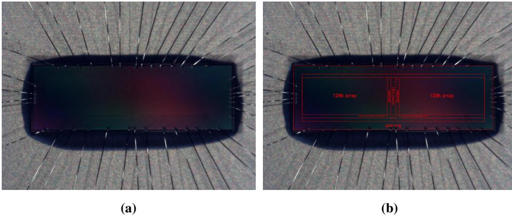
**Figure 7.3:** Photography of the stand alone 128 kbit device (a) and highlighting of the functional blocks (a).
