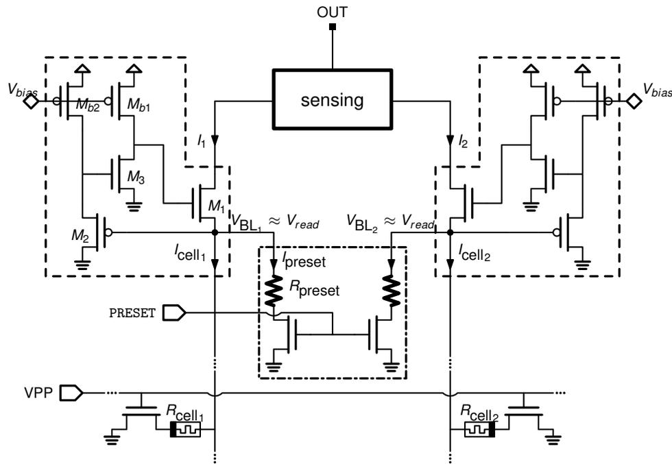
**Figure 6.23:** Schematic of the read circuit. The voltage regulators (in the dashed boxes) drive a voltage to the respective bit-lines, so that the cell currents  $I_{\text{cell}1}$  and  $I_{\text{cell}2}$  can be eventually amplified and compared by the sensing circuit. It is also present a preset circuit (in the dash-dotted box): the PRESET signal is complementary to the word-line assertion, so that the voltage regulator is ready to drive the bit-line voltage.
