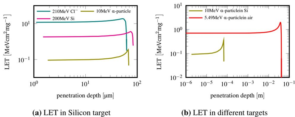
**Figure 2.1:** LET versus penetration depth for (a) different particles and (b) different targets.
