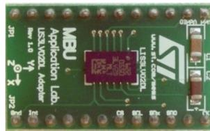
Figure 3. 7 Employed MEMS accelerometer mounted on its test board.
